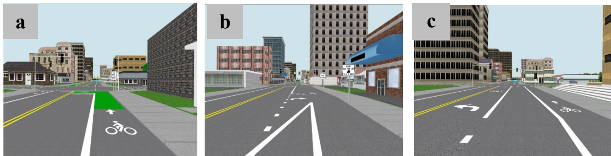
Figure 5.4: Cross-sectional geometry for (a) Bike box, (b) Mixing zone, and (c) Bicycle signal, treatments on approach to intersection
