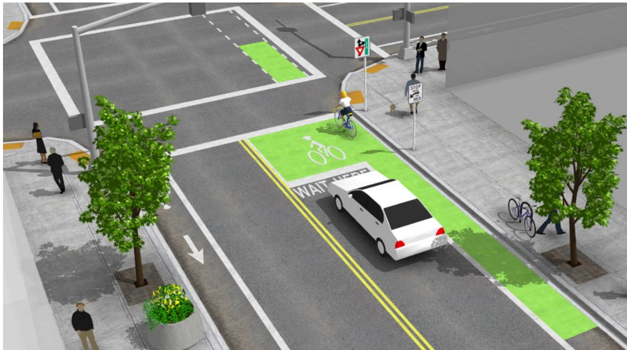
Figure 2.1: Example of a hypothetical bike box application with green paint (NACTO, 2014)
