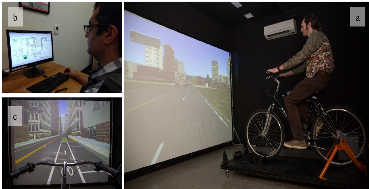
Figure 2.12: Example showing views from (a) Oregon State University bicycling simulator, (b) Operator workstation, and (c) Simulated environment (Ghodrat Abadi et al., 2019)
