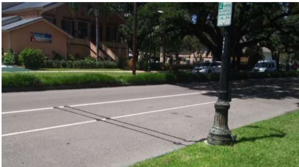
Figure 11 Esplanade Avenue count equipment configuration, outbound
