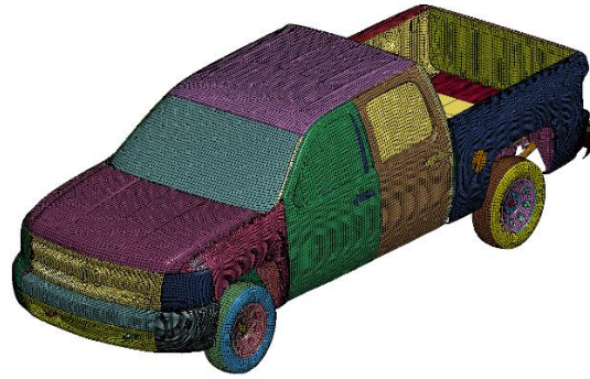
Figure 2.7. Available MASH 2270P Pickup Truck FE Model (10).
