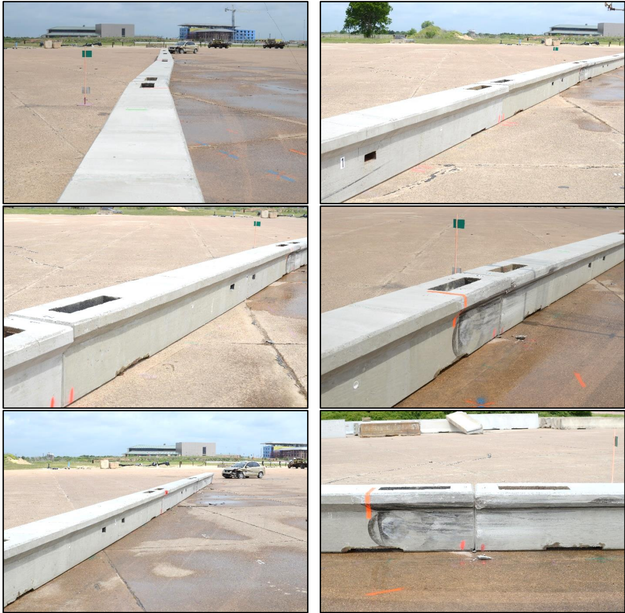
Figure 6.3. TL-3 Low-Profile Barrier after Test No. 469688-1-1.
