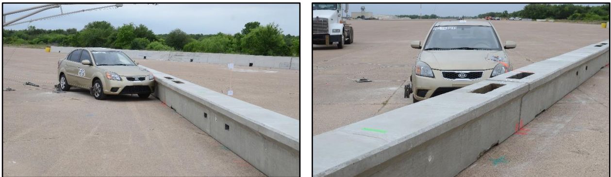
Figure 6.1. TL-3 Low-Profile Barrier/Test Vehicle Geometrics for Test No. 469688-1-1.
