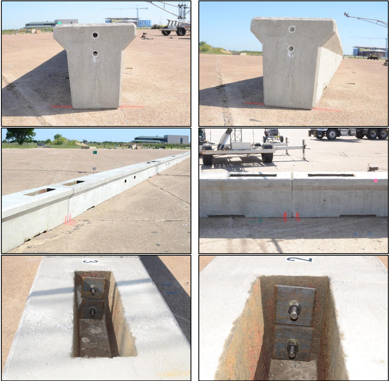
Figure 3.2. TL-3 Low-Profile Barrier prior to Testing.
