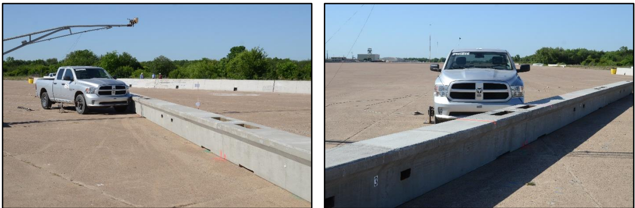
Figure 7.1. TL-3 Low-Profile Barrier/Test Vehicle Geometrics for Test No. 469688-1-2.
