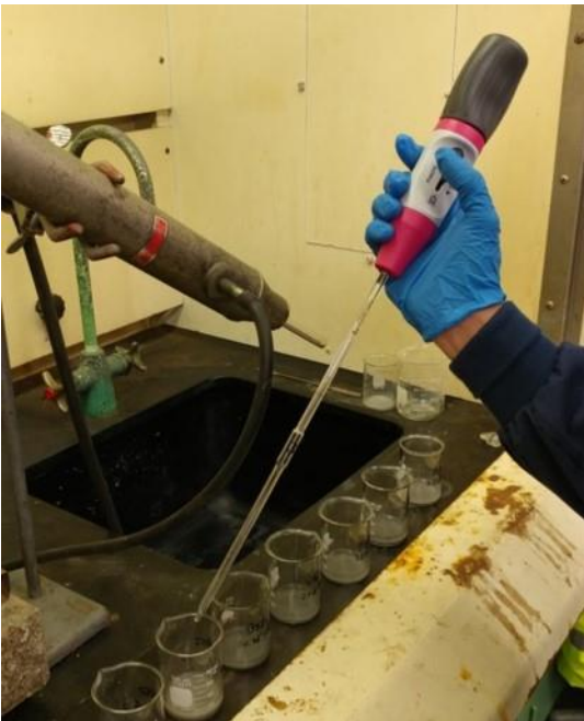
Figure 2a: Adding nitric acid
