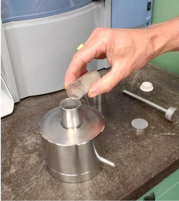
Figure 6: Creating pressed pellet
