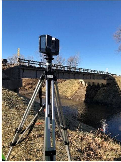
Figure 3.21: Lidar scanner used at the Hooper site.
