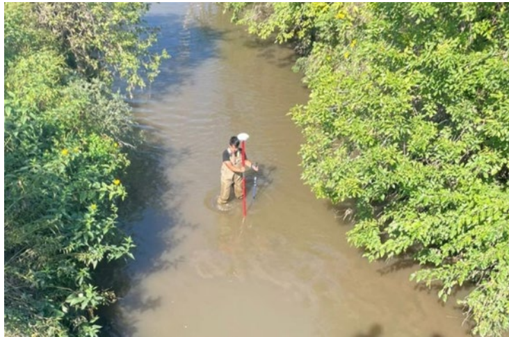
Figure 3.30: On-site GNSS-RTK data collection.
