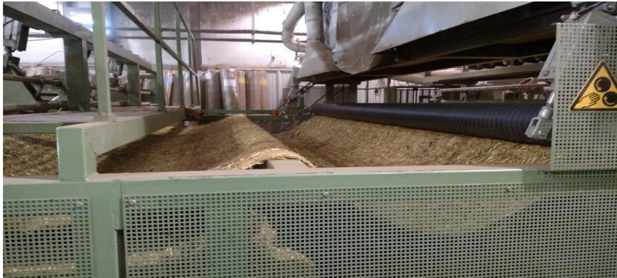
Figure 1. View of manufacturing machinery producing a rolled erosion control blanket at Ero-Guard, Inc. facility in Marshall, MN.
