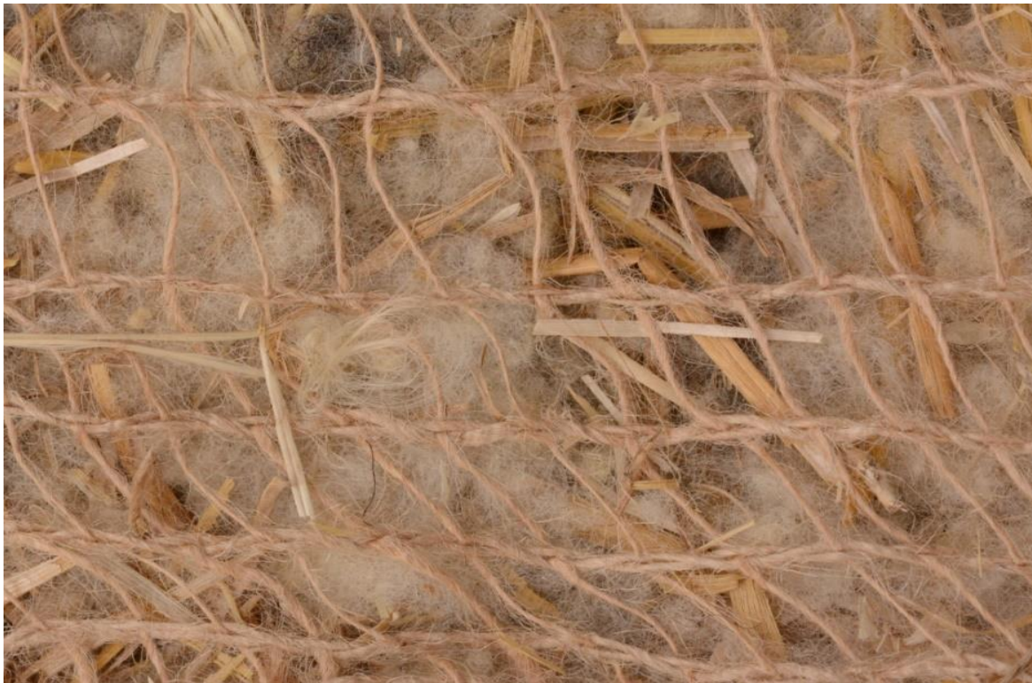
Figure 3. Close up image of an erosion control blanket showing the straw and wool fill material under the jute netting.
