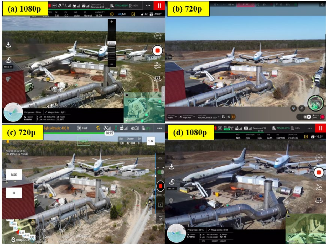
Figure 12. Comparison of Live-Streamed Visual Camera Footage: (a) M210 with Z30 Payload, (b) Parrot Anafi USA, (c) M210 with XT2 9-mm Payload, and (d) M2ED
