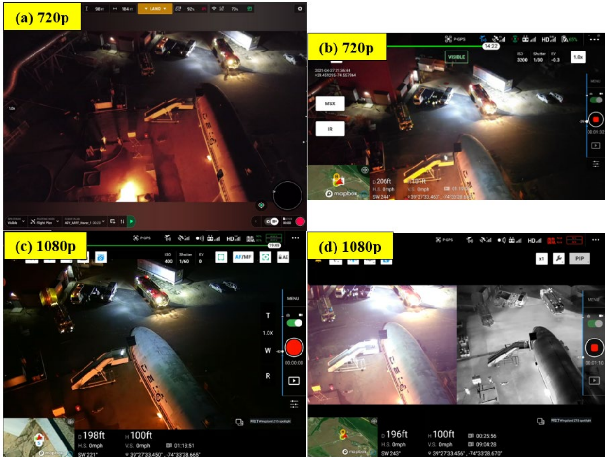
Figure 22. Nighttime Comparison of Live-Streaming Performance: (a) Parrot Anafi USA, (b) DJI M2ED, (c) DJI M210 with Z30, and (d) DJI M210 with XT2 13mm
