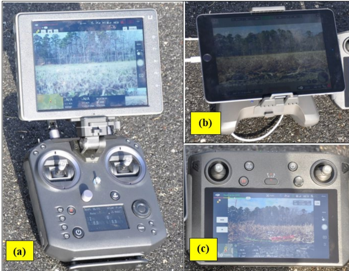
Figure 6. Ground Control Stations: (a) DJI Cendence Controller and CrystalSky Display, (b) Parrot Skycontroller 3 and iPad Mini®, and (c) DJI Smart Controller
