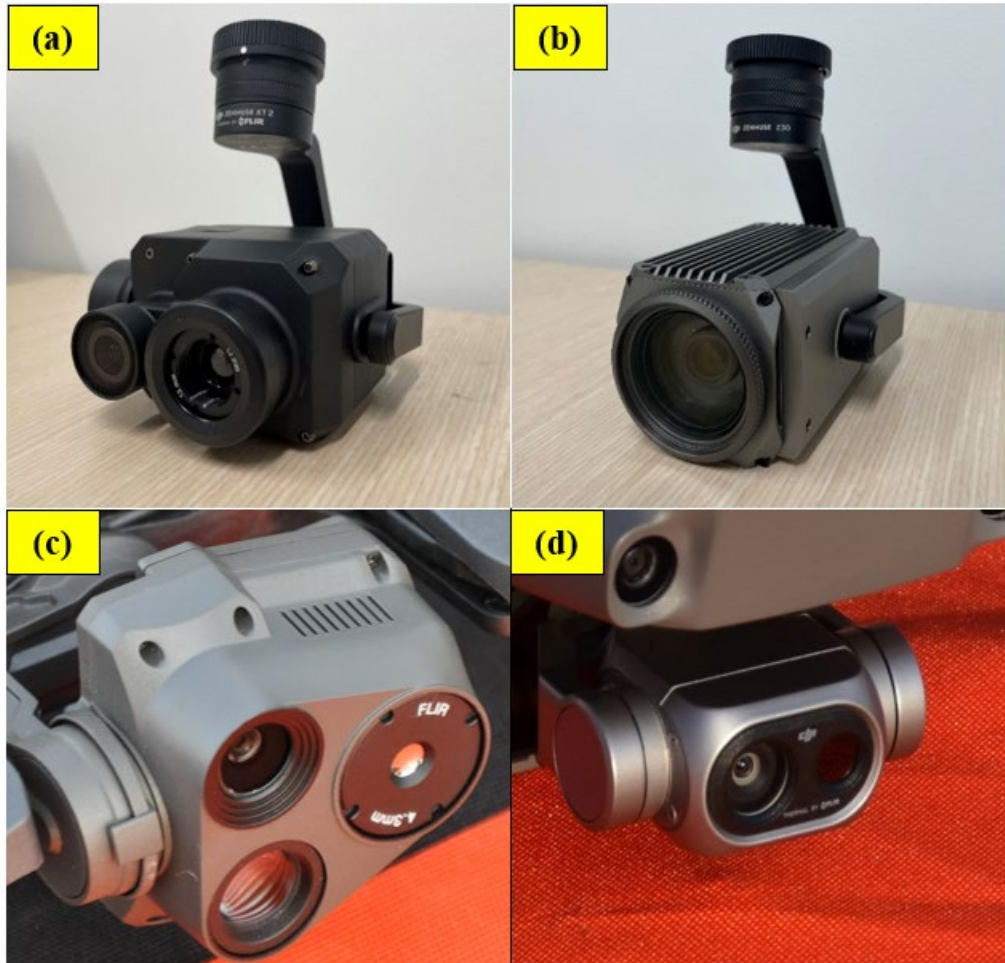
Figure 7. UAS Camera Payloads: (a) DJI Zenmuse XT2, (b) DJI Zenmuse Z30, (c) Anafi USA Triple, and (d) M2ED Integrated Camera
