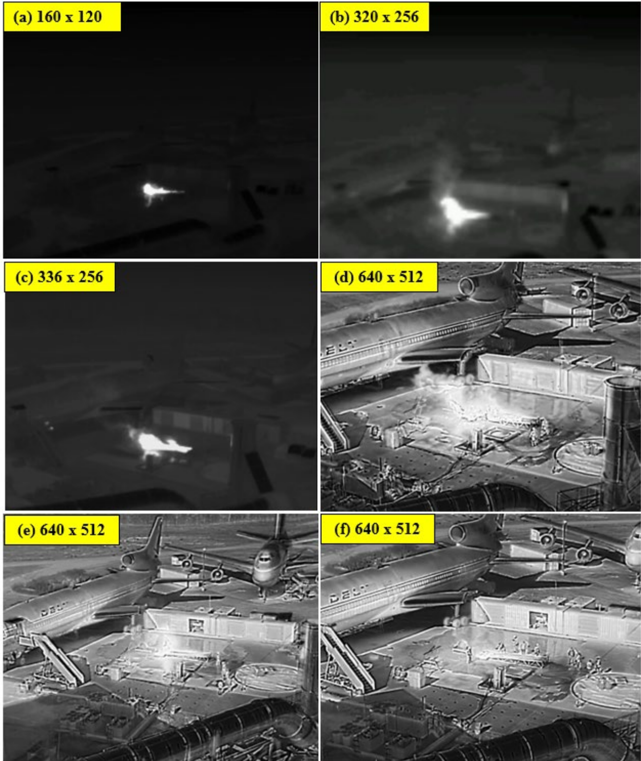
Figure 14. Comparison of Recorded Thermal Camera Performance: (a) M2ED, (b) Anafi Triple, (c) XT2 9mm, (d) XT2 13mm, (e) XT2 19mm, and (f) XT2 25mm
