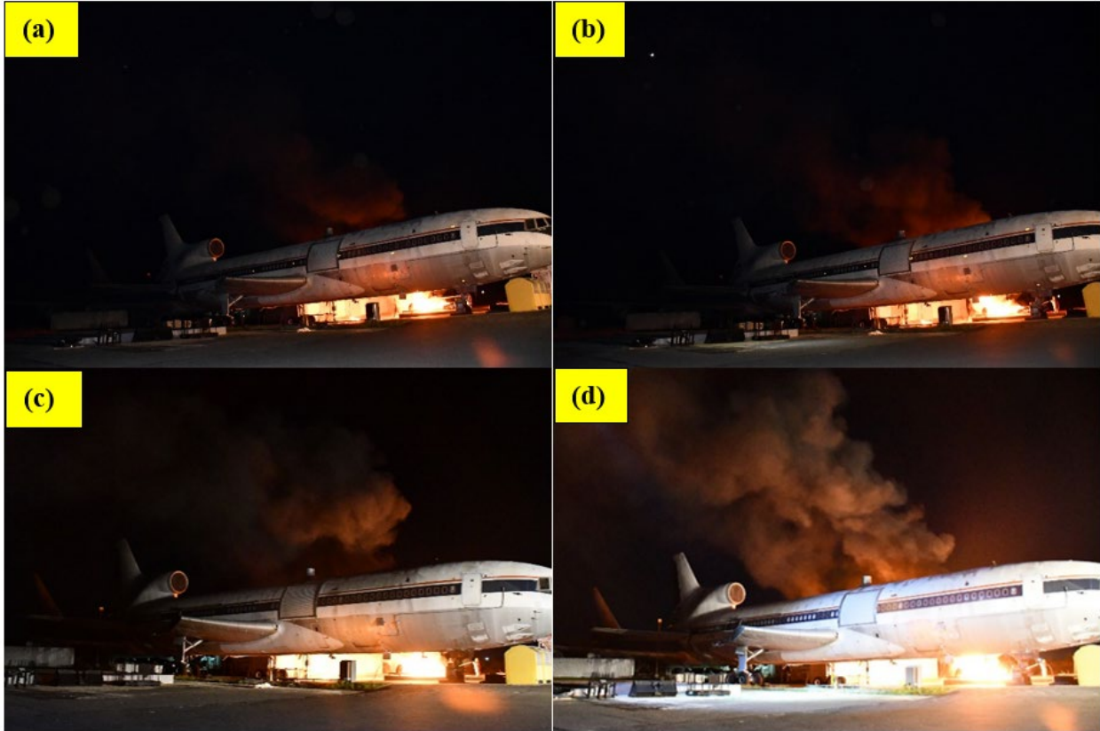
Figure 30. Comparison of Spotlight Payload Efficacy from the Ground: (a) M2ED Spotlight Off, (b) M2ED Spotlight On, (c) M210 Spotlight Off, and (d) M210 Spotlight On
