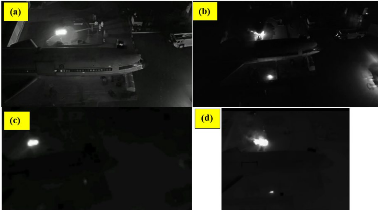
Figure 28. Nighttime Comparison of Blended Footage with Thermal Camera Footage: (a) M2ED Blended, (b) Anafi Triple Blended, (c) M2ED Thermal, and (d) Anafi Triple Thermal
