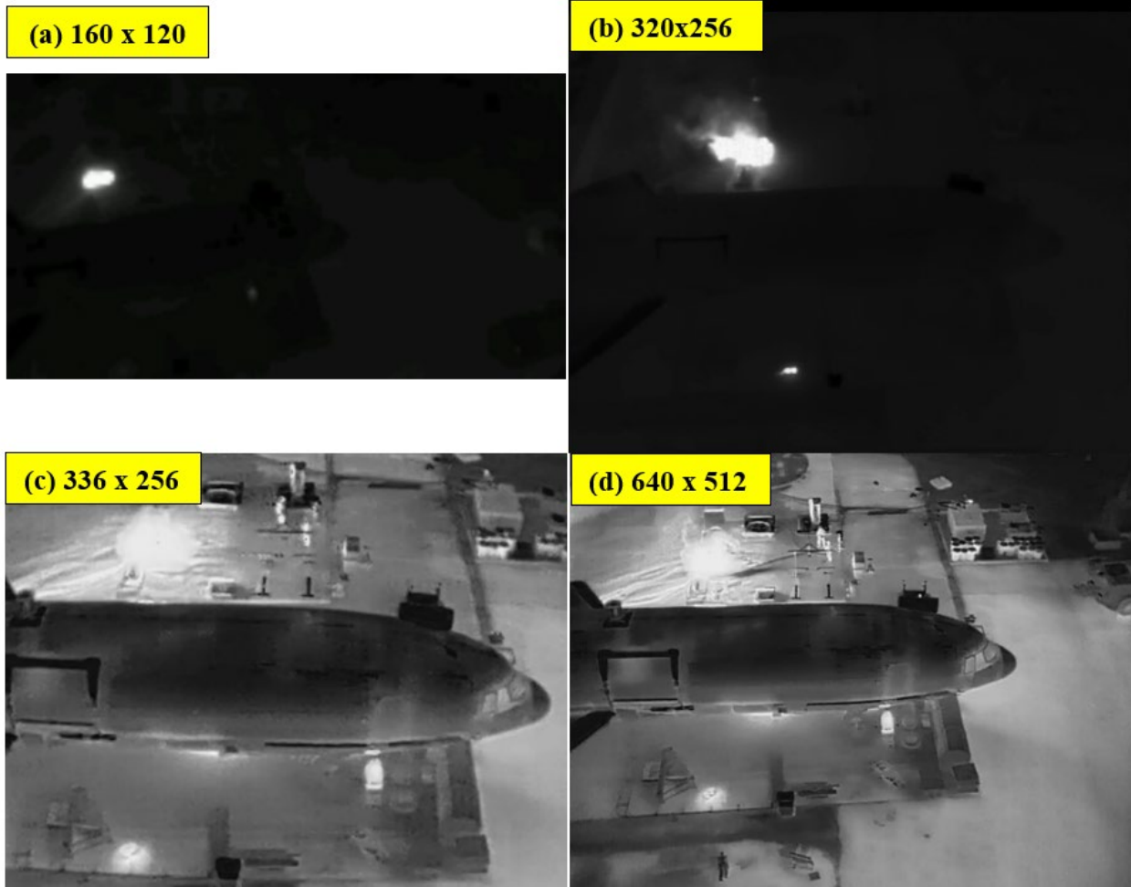
Figure 27. Nighttime Comparison of Recorded Thermal Camera Footage: (a) M2ED, (b) Anafi Triple, (c) XT2 9mm, and (d) XT2 13mm
