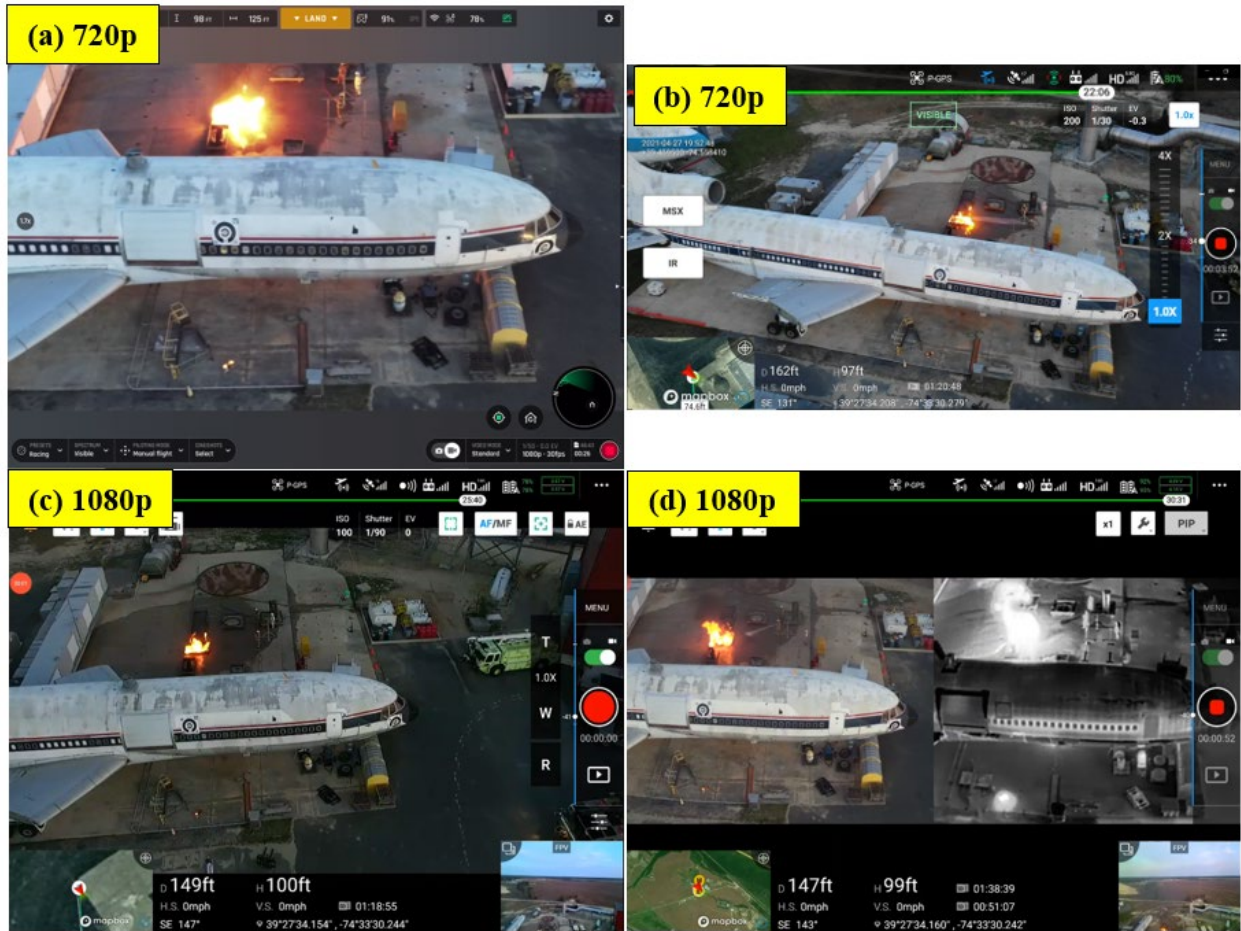
Figure 21. Twilight Comparison of Live-Streaming Performance: (a) Parrot Anafi USA, (b) DJI M2ED, (c) DJI M210 with Z30, and (d) DJI M210 with XT2 13mm
