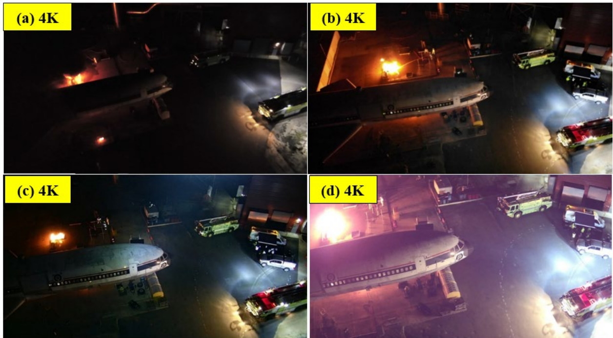
Figure 25. Nighttime Comparison of Recorded Visual Camera Footage: (a) Anafi Triple, (b) M2ED, (c) Z30, and (d) XT2 9mm
