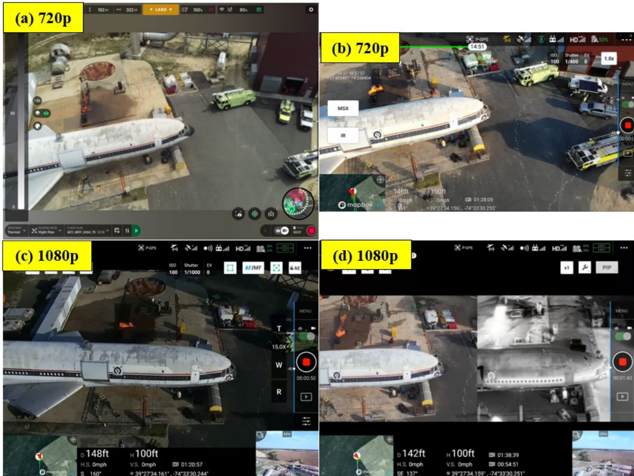
Figure 20. Daylight Comparison of Live-Streaming Performance: (a) Parrot Anafi USA, (b) M2ED, (c) M210 with Z30 Payload, and (d) M210 with XT2 13mm Payload
