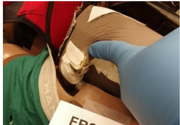
Figure I-31. Damage to the THOR-50M ABISUP Abdomen During Test V10-3: All Damage Was Minor, and Was Related to Seams and Corners of the ABISU
