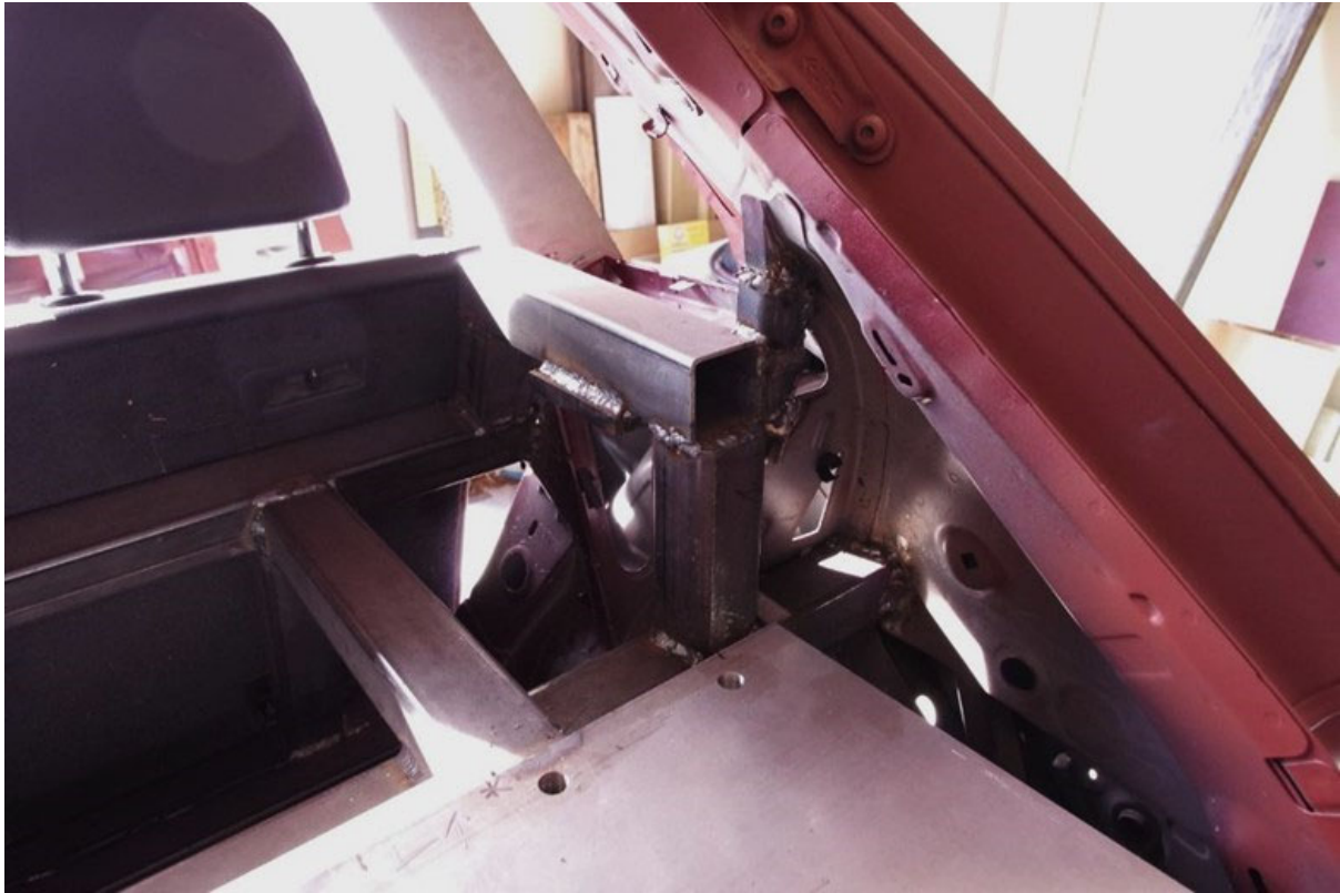
Figure A-7. Rear Seat and Retractor Reinforcement of the VI Buck
