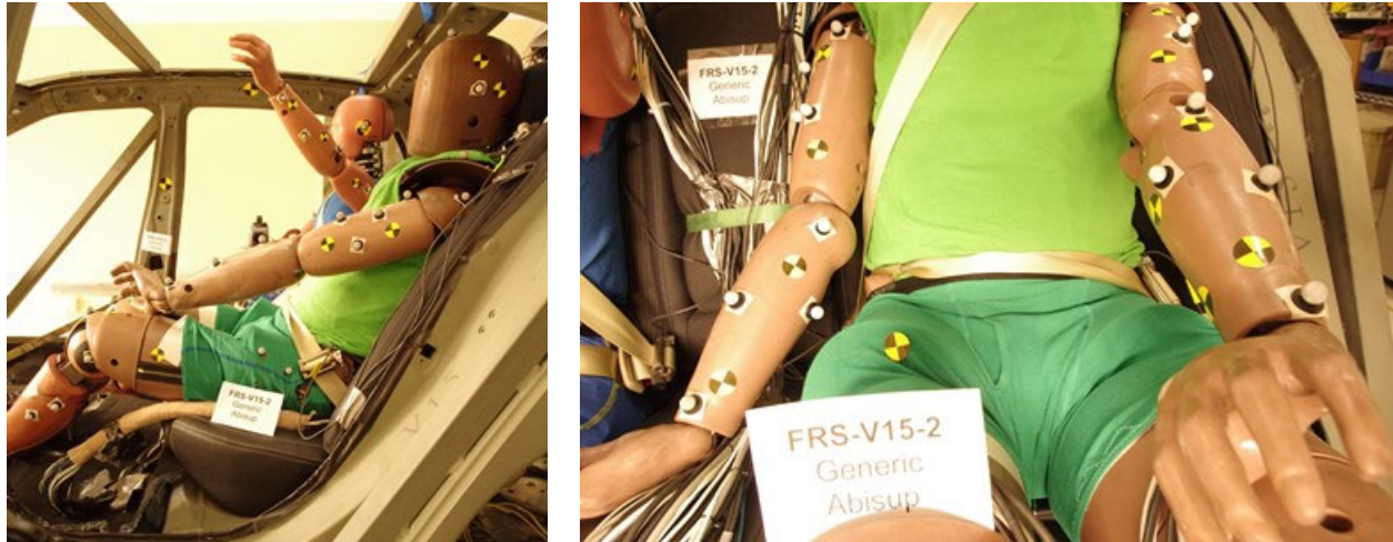
Figure 4-36. Post-Test Pictures of Test FRS-V15-2, Which Involved Minor Submarining of the THOR Dummy With the Belt Penetrating the Abdomen on the Right (Inboard) Side
