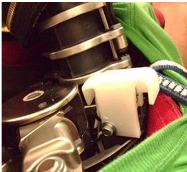
Figure I-21. The THOR-50M T1 Accelerometer Mount and Shroud Were Damaged During Test V6-4: The Mount Locating Pin and Retaining Bolt Were Compromised
