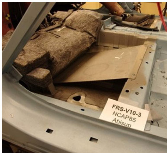
Figure I-28. Ramps Installed for Both ATDs in Buck V10 Prior to Test V10-3: These Ramps Were Designed to Prevent Contact Between the Dummy Toes and the Front Seat Riser
