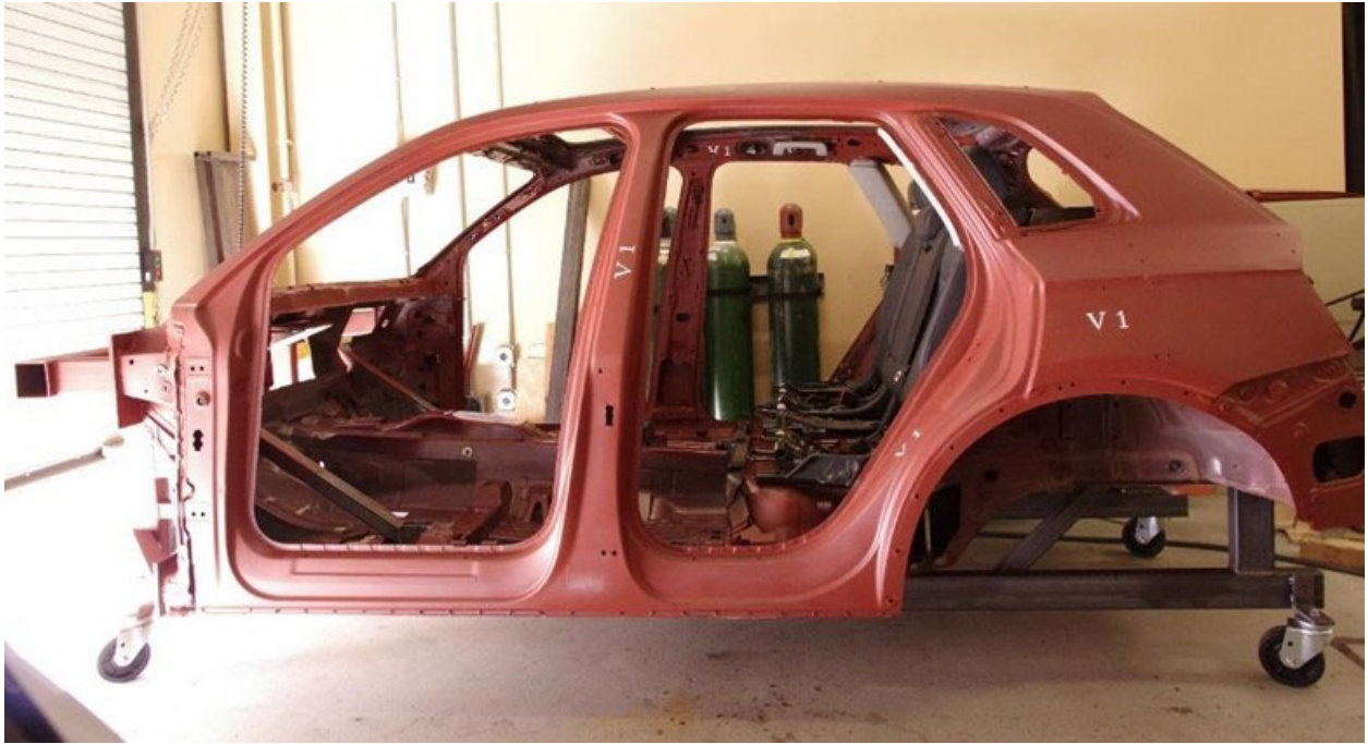
Figure A-1. The Completed V1 Buck on Casters
