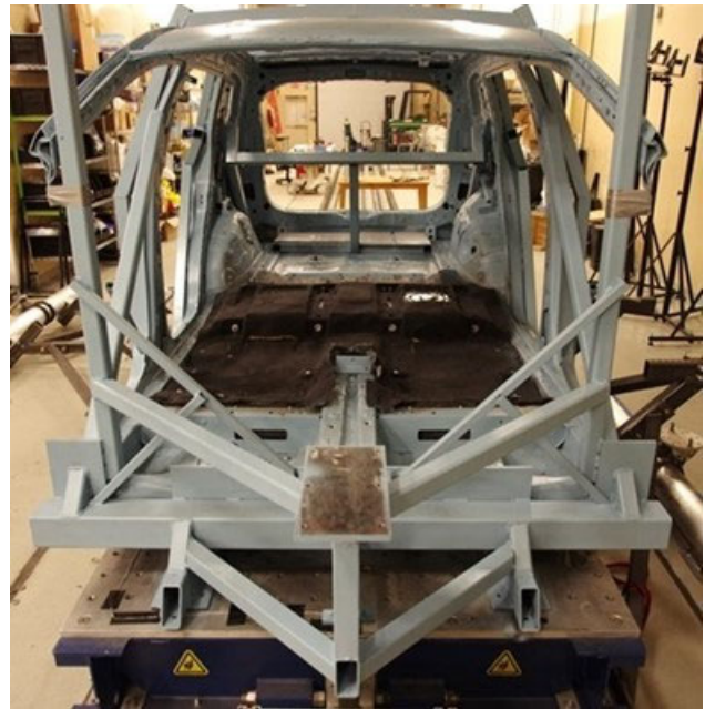
Figure C-2. Front Reinforcement Structure Detail of the V10 Buck
