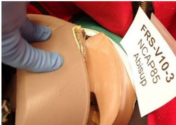
Figure I-31. Damage to the THOR-50M ABISUP Abdomen During Test V10-3: All Damage Was Minor, and Was Related to Seams and Corners of the ABISU
