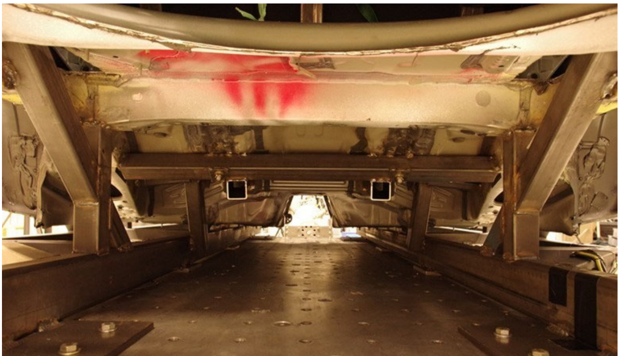
Figure G-4. Underside of the V19 Buck Showing Rear Supports
