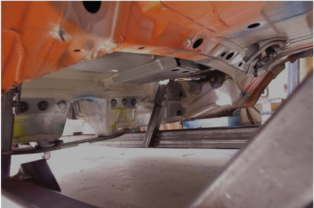
Figure A-4. Underside of the V1 Buck Showing Detachable Seat Track and Frame Support
