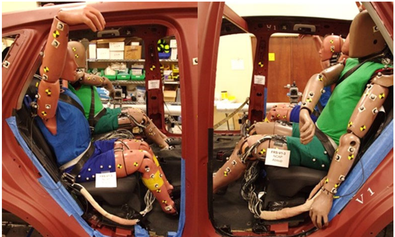
Figure J-6. Post-Test Images for Vehicle V1, Test 3 (NCAP85 Pulse)
