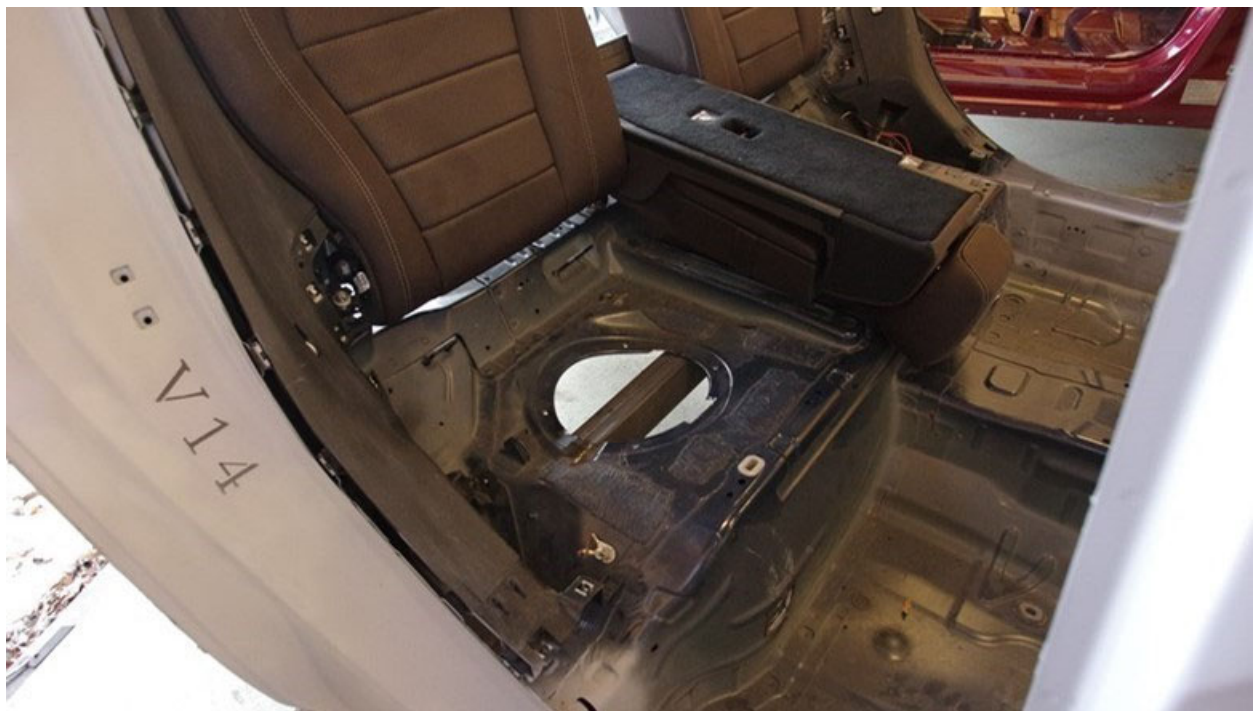
Figure E-6. Detail of the V14 Buck Seat Pan Reinforcement From Above
