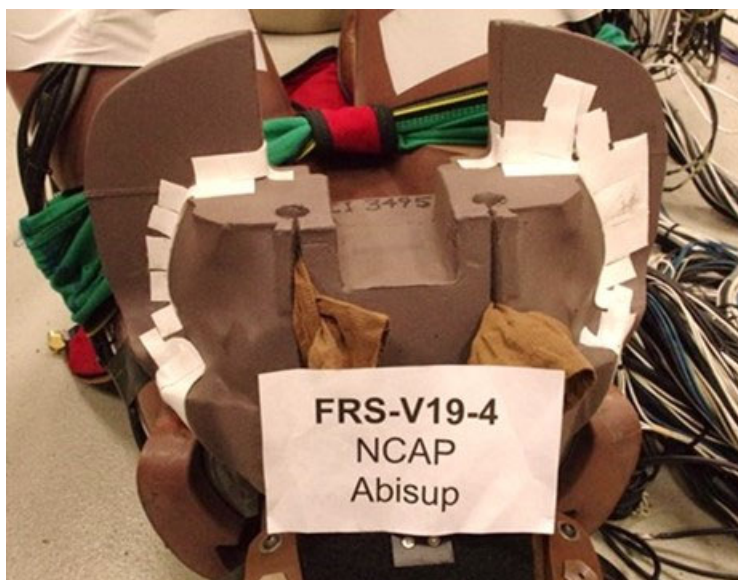
Figure I-40. Collection of Robust Repairs Made to the THOR-50M ABISUP Between Tests: Damage Typically Occurred at the Seams and Corners of the ABISUP
