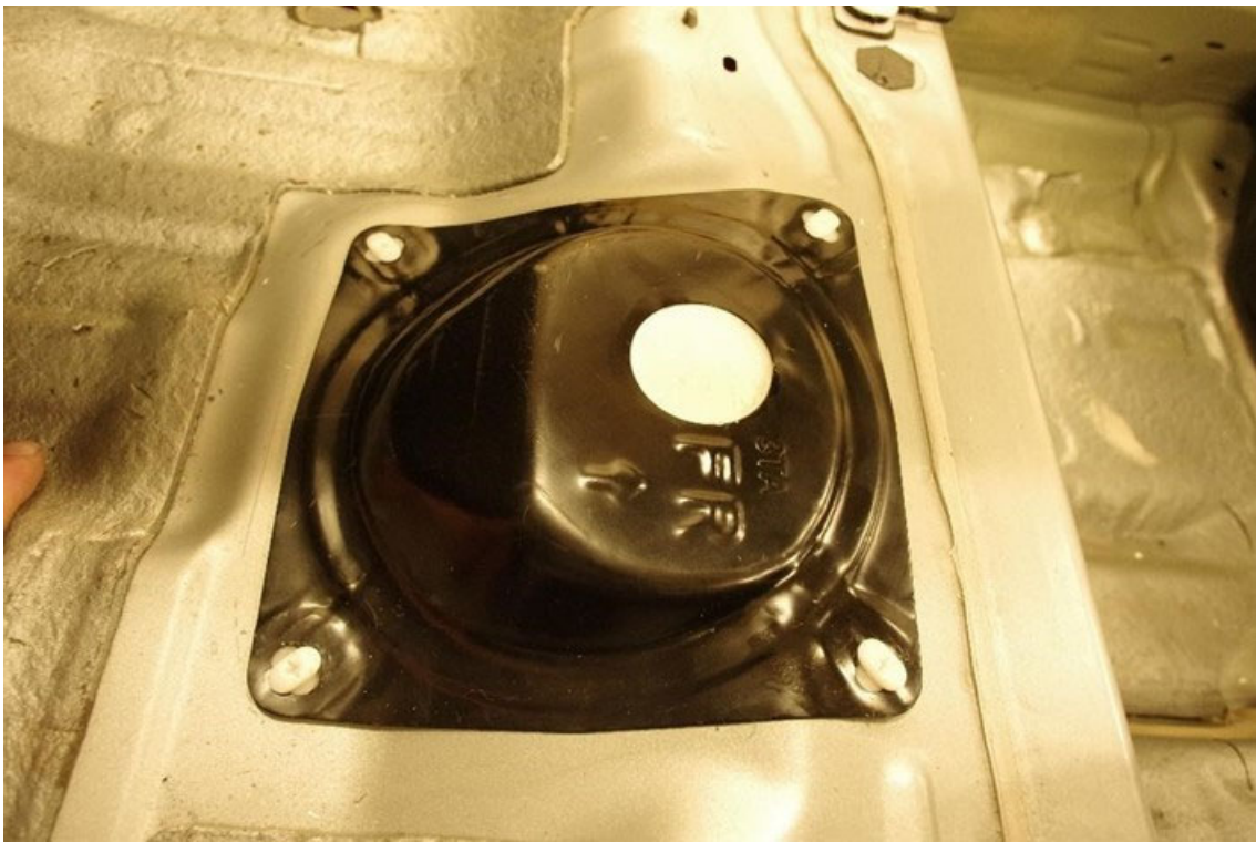
Figure F-8. Urethane Foam Support of the Fuel Tank Access Cover
