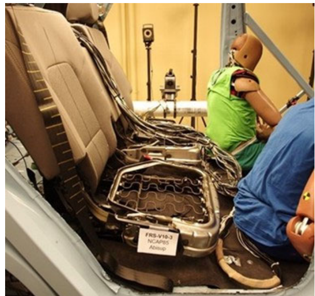
Figure I-32. Seat Bottom Damage From Test V10-3
