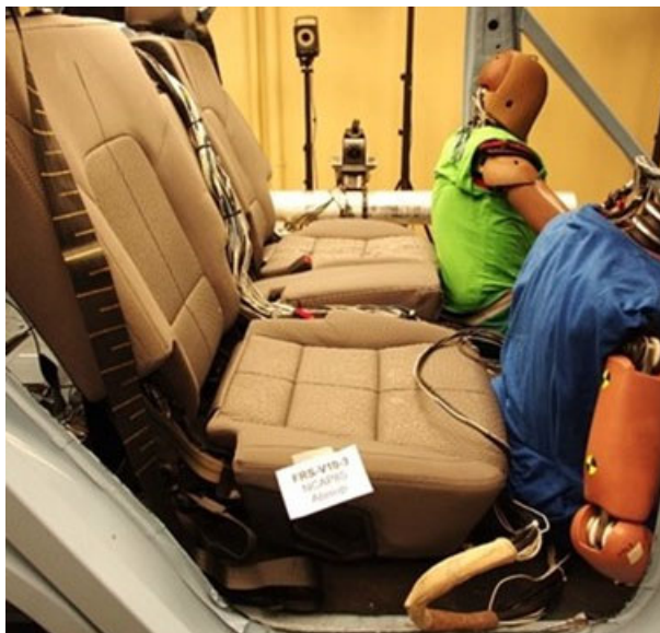
Figure I-32. Seat Bottom Damage From Test V10-3
