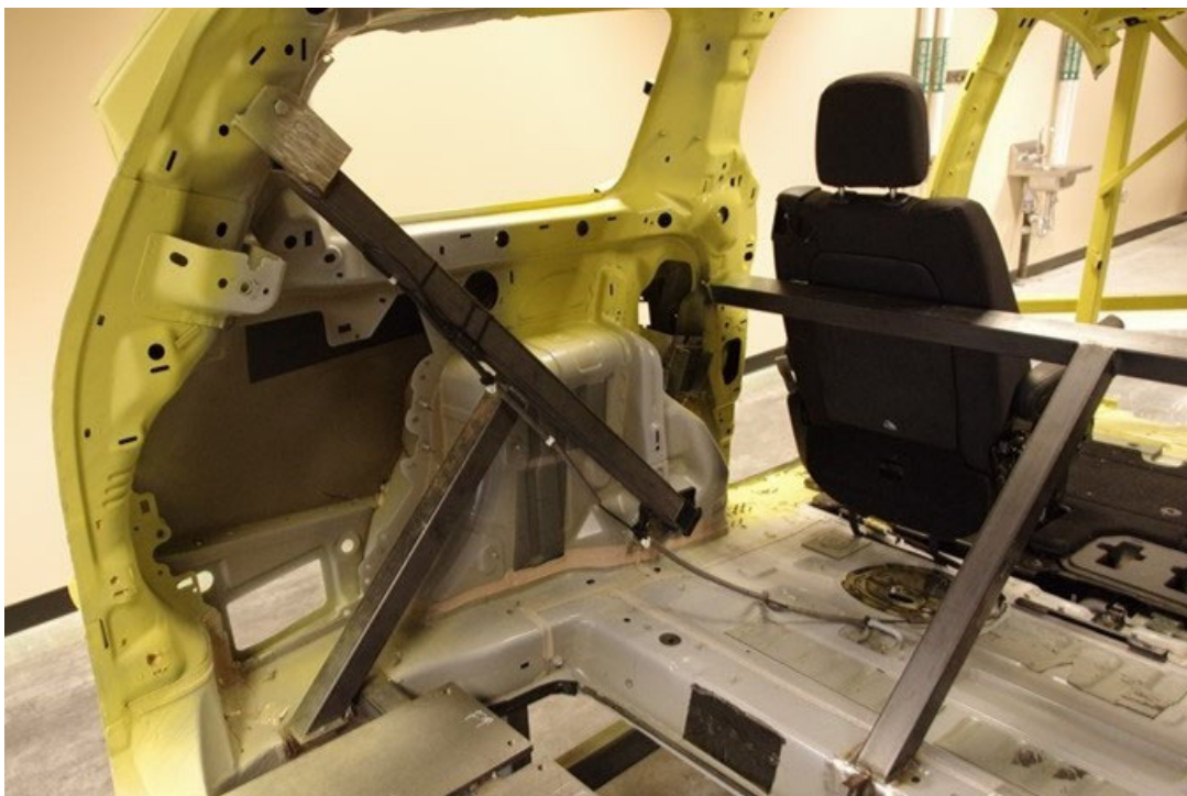
Figure B-4. Internal V6 Buck Rear Structural Detail
