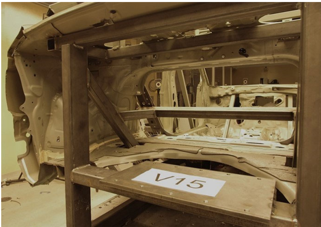
Figure F-4. Posterior Oblique View of the V15 Buck on the Sled Showing Seatback Reinforcement and DAS Mounting Plates
