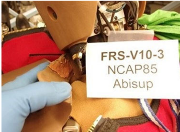
Figure I-30. Damage to the THOR-50M Collar Repair From Test V10-3
