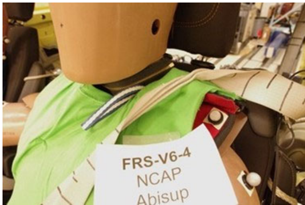
Figure I-20. During Test V6-4 the Shoulder Belt Folded Over on Itself as It Was Trapped by the Shoulder of THOR-50M
