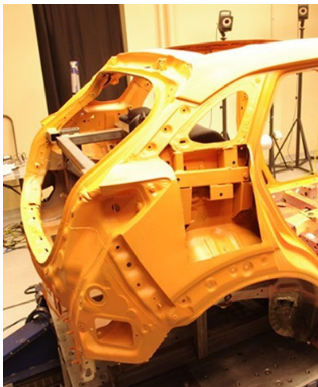
Figure D-4. Detail of the Rear Seat and Retractor Reinforcement on the V13 Buck
