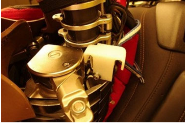
Figure I-14. THOR-50M T1 Accelerometer Mount Shroud Installed for Test V-4: It Was Designed to Keep the T1 Mount From Cutting the Shoulder Belt
