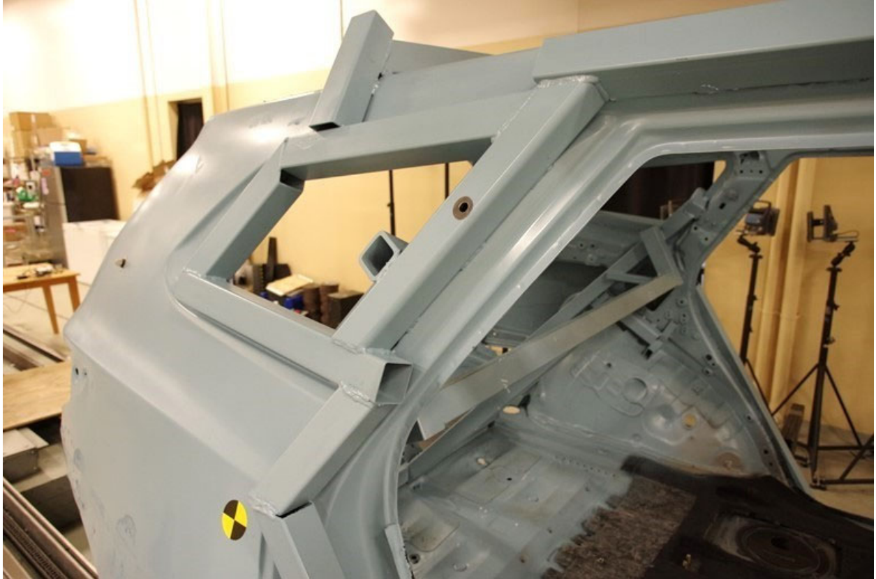
Figure C-5. Exterior Detail of Rear Structural Reinforcement and Restraint Support
