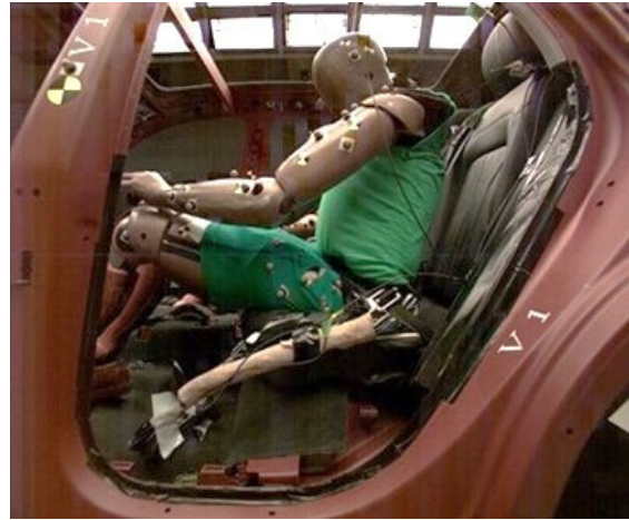
Figure PP-1. Test FRS-V1-1 HIII (Left) and THOR (Right) at Peak Hip Excursion
