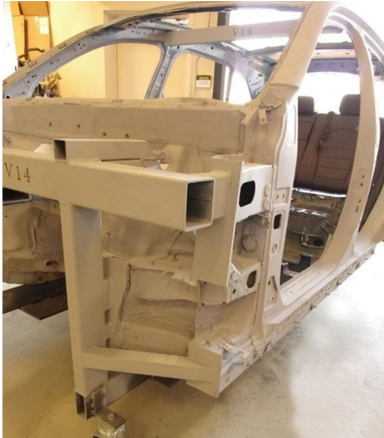
Figure E-3. Front Reinforcement Detail of the V14 Buck
