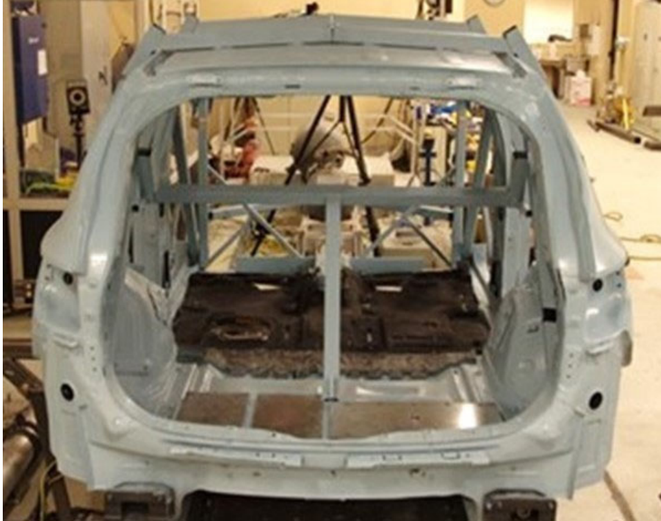
Figure C-3. Rear Reinforcement Structure and Seat Support in the V10 Buck
