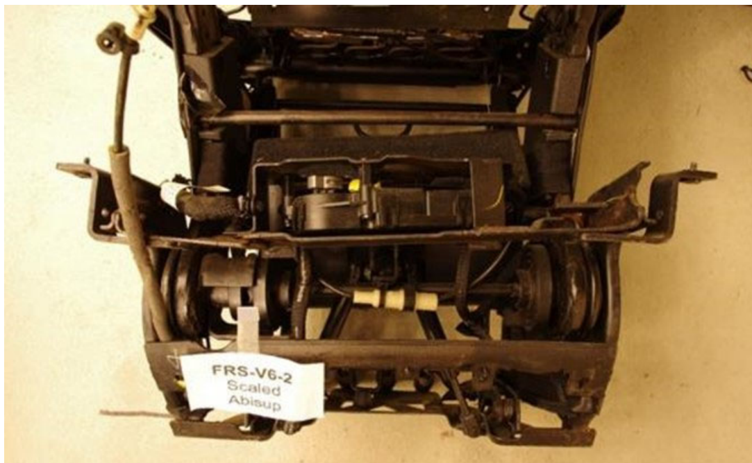
Figure I-5. Test V6-2 THOR-50M Seat Pedestal Mounting Bracket Separated and Deformed: The Pedestals for Both ATDs Were Realigned and Reinforced by Welding for Test V6-3
