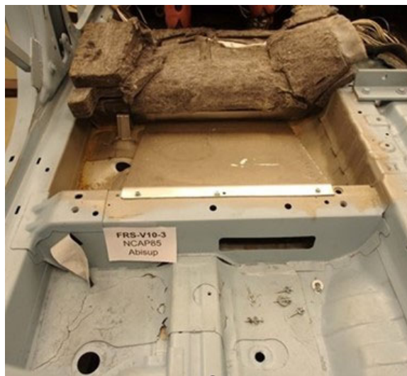
Figure I-28. Ramps Installed for Both ATDs in Buck V10 Prior to Test V10-3: These Ramps Were Designed to Prevent Contact Between the Dummy Toes and the Front Seat Riser
