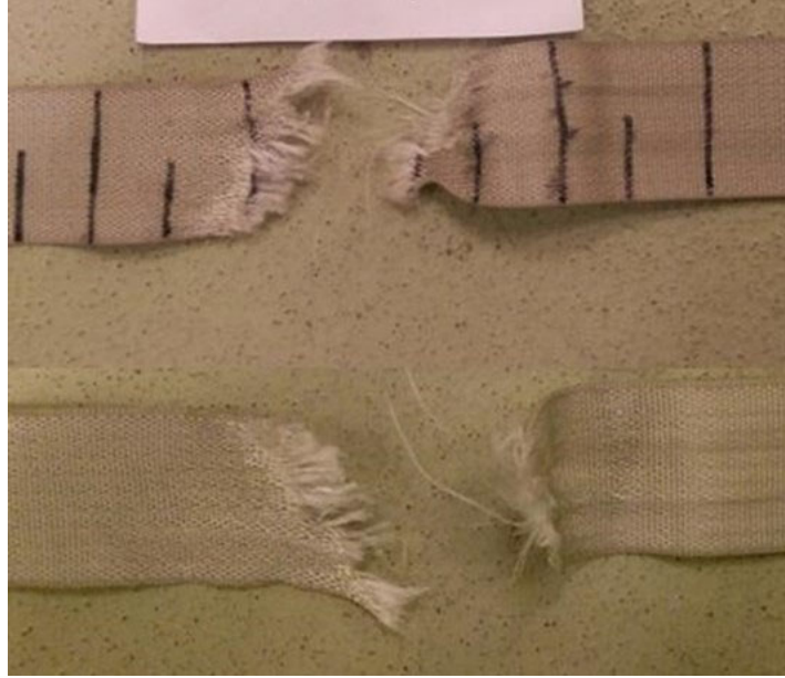
Figure I-7. Test V6-3 Torn Shoulder Belt (Both Sides Shown) for the THOR-50M: The Belt Was Torn During Interaction With the T1 Accelerometer Mount and the Z-Direction Accelerometer Was Damaged
