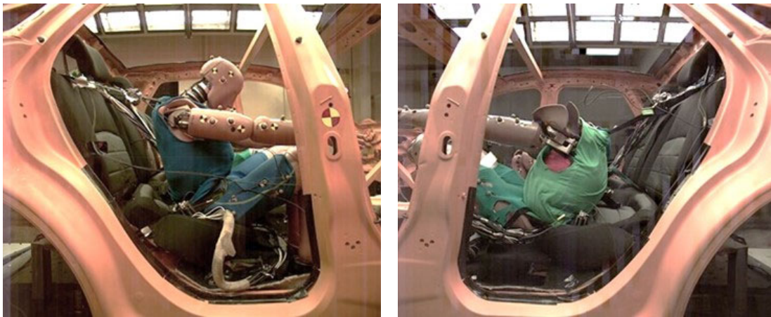
Figure RR-5. Test FRS-V13-2 HIII (Left) and THOR (Right) at Peak Hip Excursion
