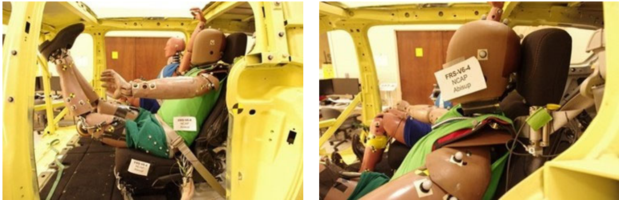
Figure I-18. Post Test V6-4 THOR-50M Posture: The Shoulder Belt Slipped Between the Neck and Shoulder but Did Not Get Cut, and the Knees Did Not Over-Rotate Appreciably
