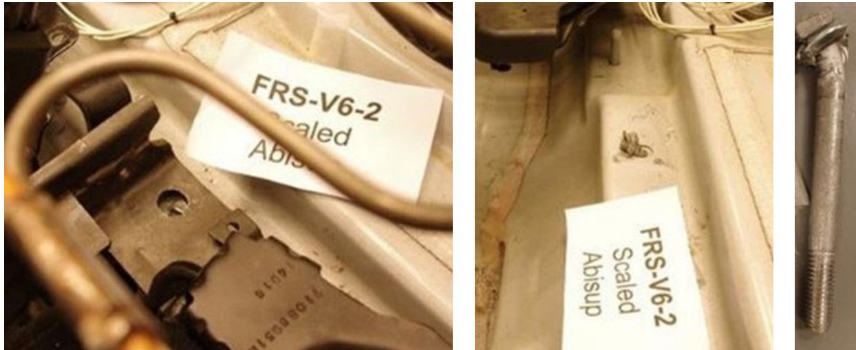
Figure I-4. Test V6-2, THOR-50M Inboard Rear-Seat Pedestal Anchor Pulled Through Bracket (Left), Deformed Anchor Bolt and Washer in Pedestal Riser (Middle), and Deformed Anchor Bolt and Washer in Pedestal Riser (Right): A Grade 9 Bolt Was Used for Test V6-3, and a Small Plate Was Used Instead of a Washer
