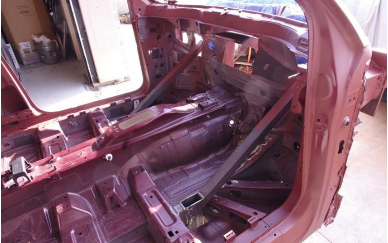
Figure A-10. Reinforcement of the Interior Front of the V1 Buck.
