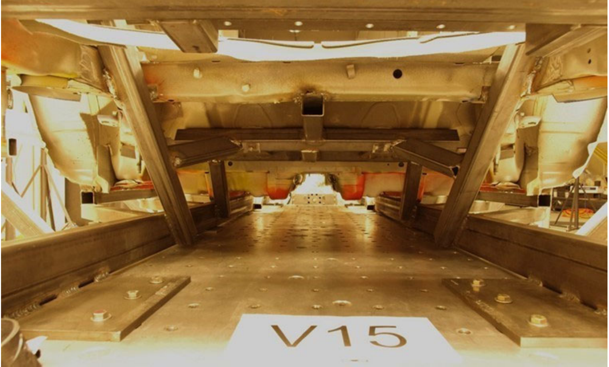
Figure F-5. Underside of the V15 Buck on the Sled
