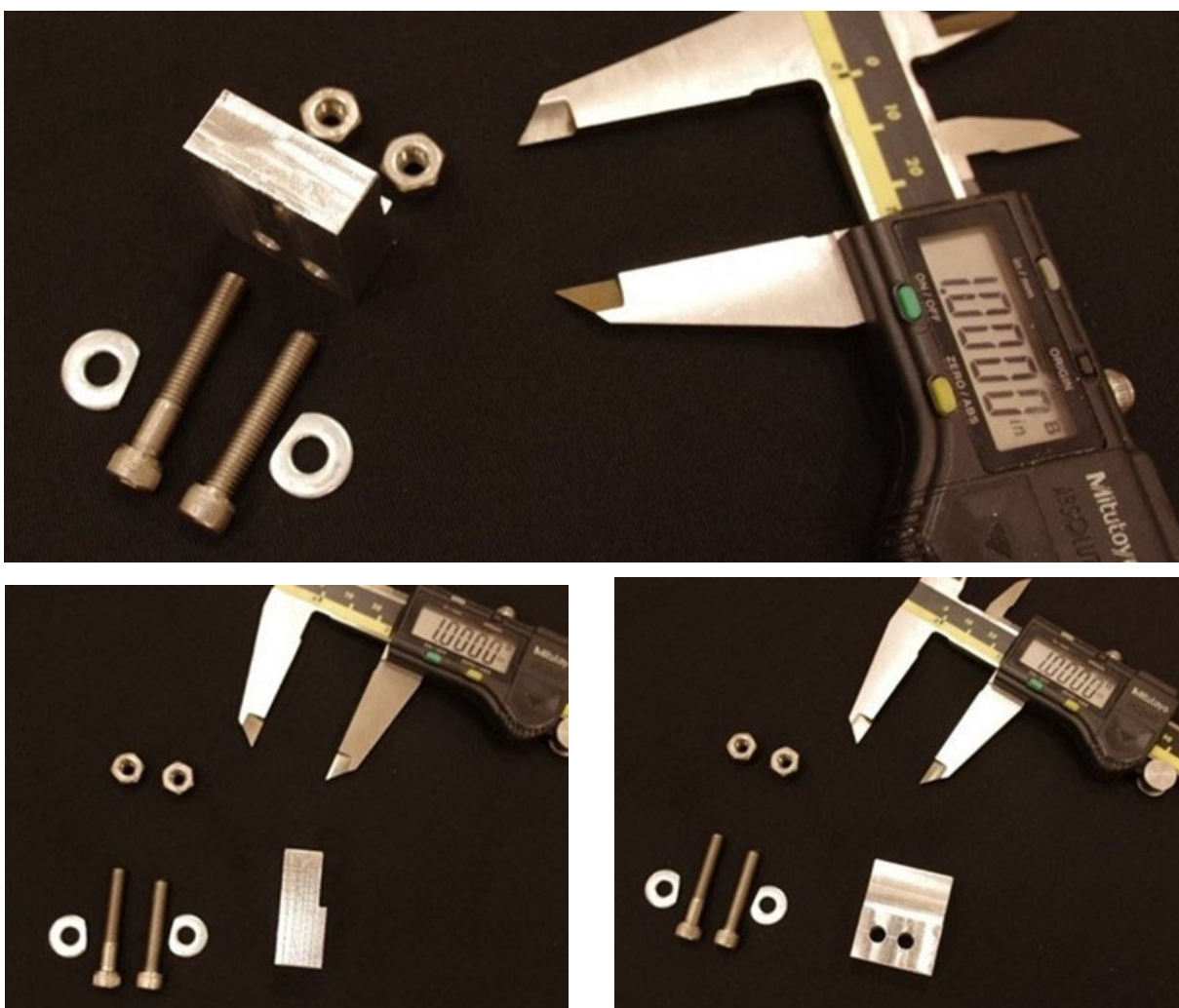
Figure I-23. Different Perspectives of the Locating Block Used to Position the T1 Accelerometer Mount on the Right Side of the THOR-50M Without Any Pins: This Block Was Used for All V10 Tests
