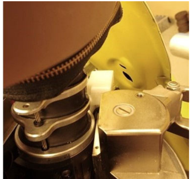
Figure I-15. The THOR-50M T1 Accelerometer Mount Shroud Protects the Shoulder Belt When It Slips Between the Neck and Shoulder
