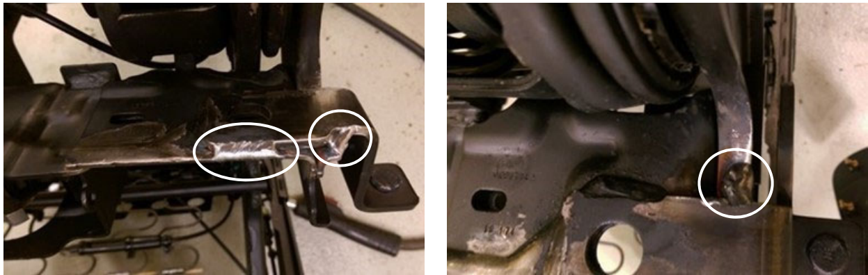
Figure I-11. New Seat Pedestals and Reinforcing Weldments Used for Test V6-4 for Both ATDs
