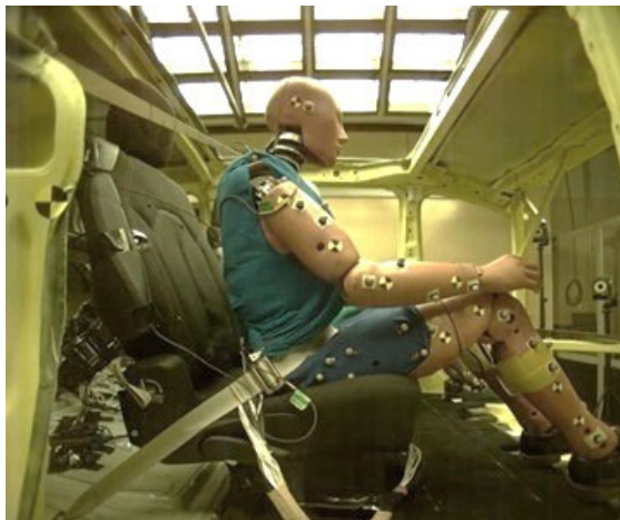
Figure PP-2. Test FRS-V6-1 HIII (Left) and THOR (Right) at Peak Hip Excursion
