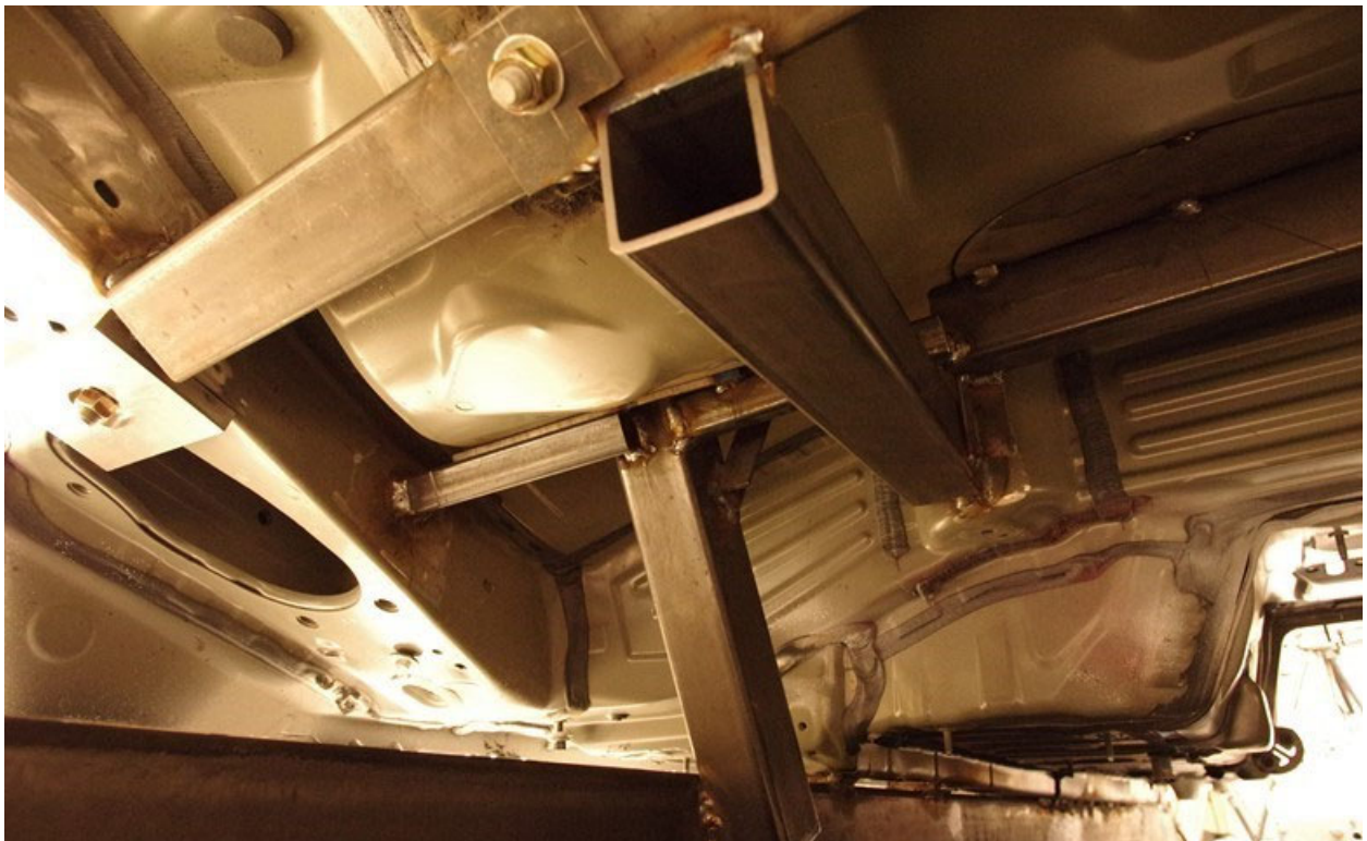
Figure G-6. Detail of Rear Anchor and Seat Support Structure on the V19 Buck
