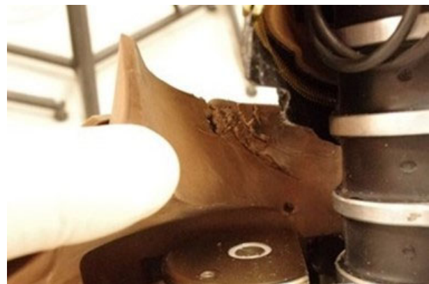
Figure I-22. THOR-50M Collar Damage From Test V6-4
