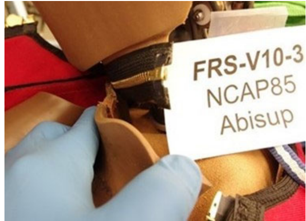
Figure I-30. Damage to the THOR-50M Collar Repair From Test V10-3
