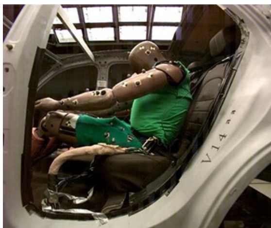
Figure PP-5. Test FRS-V14-1 HIII (Left) and THOR (Right) at Peak Hip Excursion
