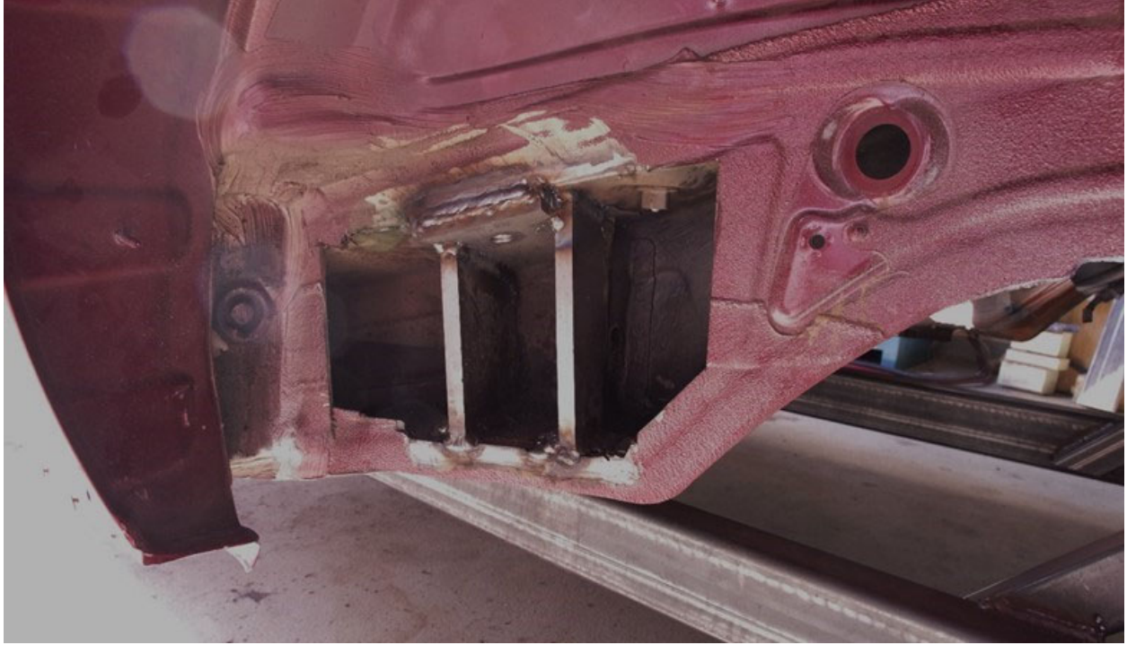
Figure A-3. Anchor Point Reinforcement Detail on the V1 Buck
