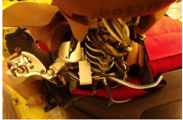
Figure I-14. THOR-50M T1 Accelerometer Mount Shroud Installed for Test V-4: It Was Designed to Keep the T1 Mount From Cutting the Shoulder Belt
