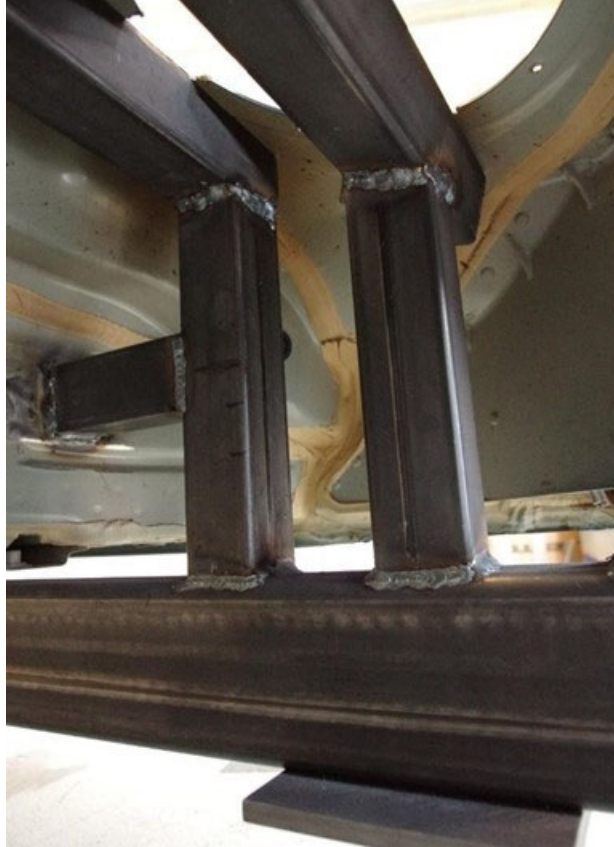
Figure E-5. Detail of the V14 Buck Seat Pan Reinforcement From Below
