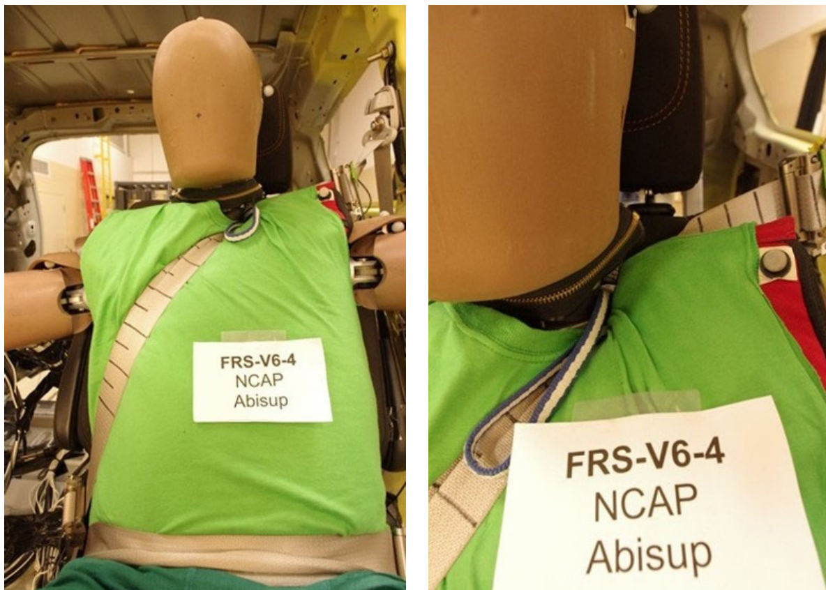
Figure I-19. During Test V6-4 the Shoulder Belt Slipped Past the Collar and Leather Bib Installed on the THOR-50M and Was Trapped Between the T1 Accelerometer Mount Shroud and the Shoulder
