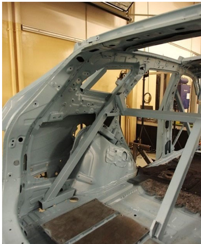
Figure C-4. Interior Detail of Rear Structural Reinforcement and Restraint Support
