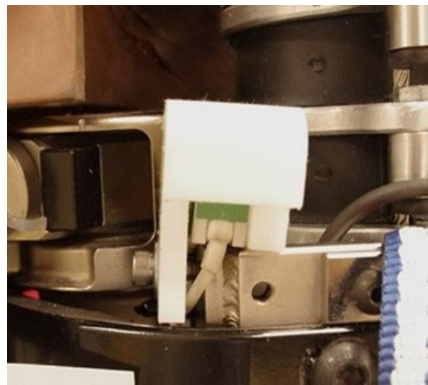
Figure I-21. The THOR-50M T1 Accelerometer Mount and Shroud Were Damaged During Test V6-4: The Mount Locating Pin and Retaining Bolt Were Compromised
