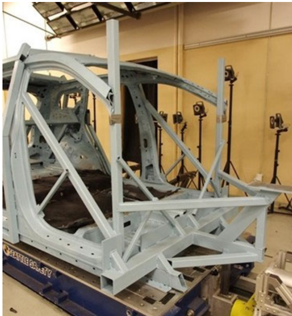
Figure C-2. Front Reinforcement Structure Detail of the V10 Buck
