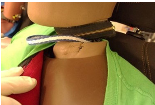
Figure I-22. THOR-50M Collar Damage From Test V6-4
