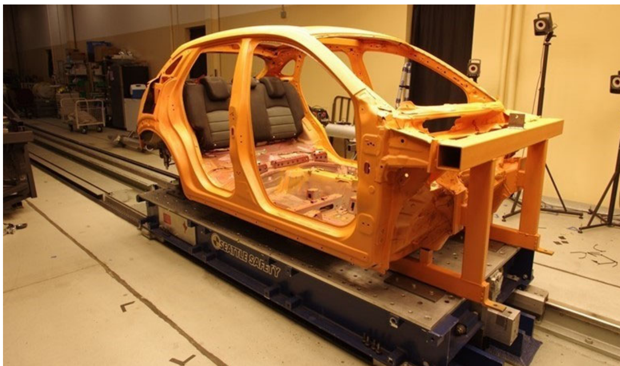
Figure D-2. Oblique Perspective of the V13 Buck on the Sled
