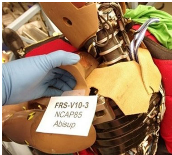
Figure I-29. The Expanded Bib Covering the Shoulder of the THOR-50M for Test V10-3 (Left), and the T1 Shroud Used to Fill the Space on the Left Side of the Dummy (Right)
