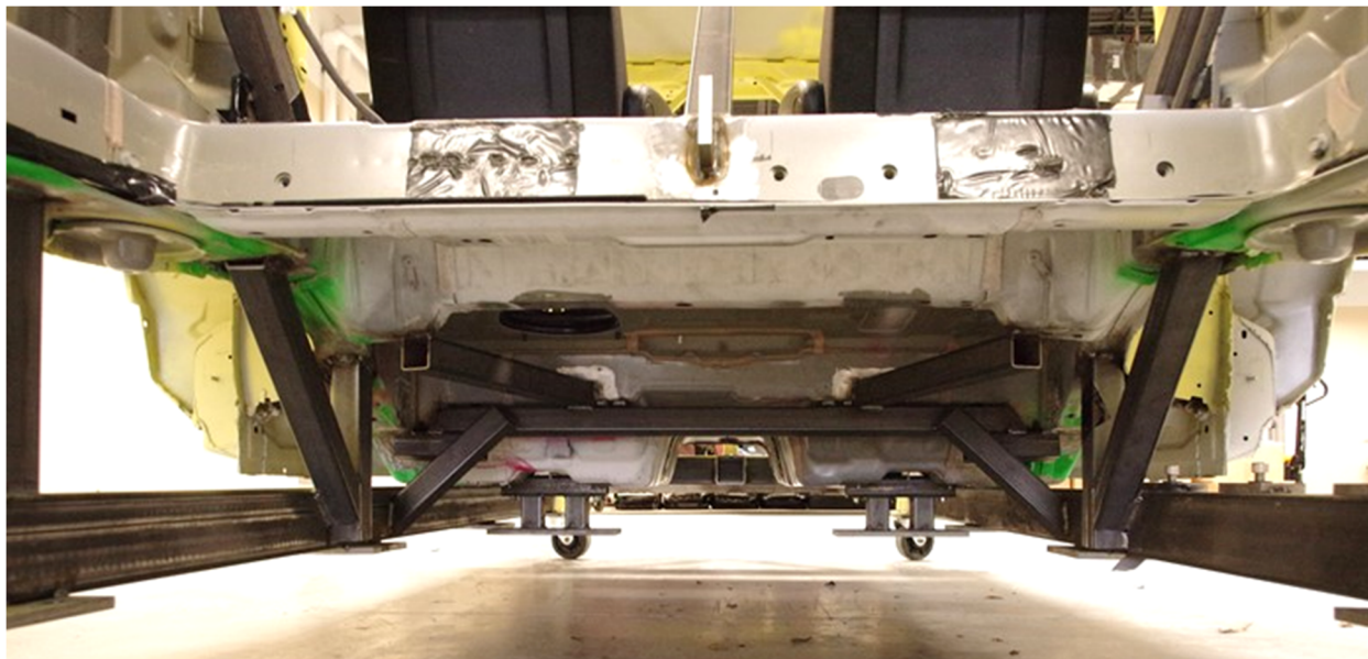
Figure B-5. Underneath V6 Buck Rear Seat and Anchor Reinforcements
