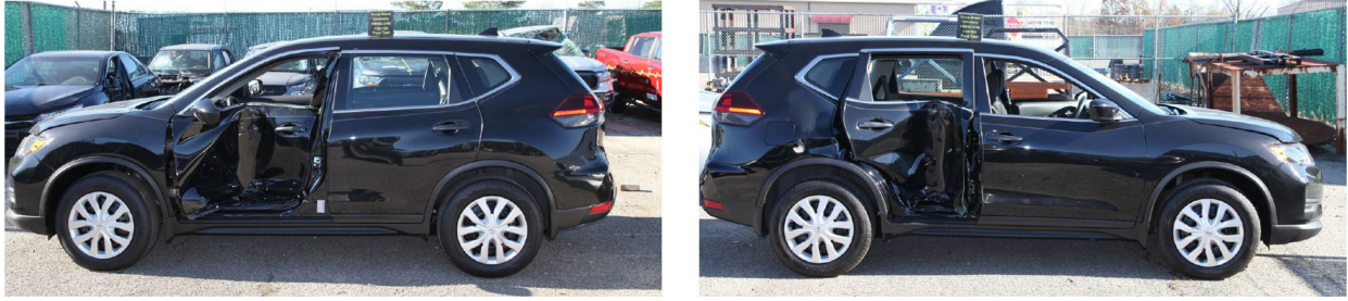
Figure 33. Nissan Rogue FMVSS No. 214 static post crash (a) front door; (b) rear door
