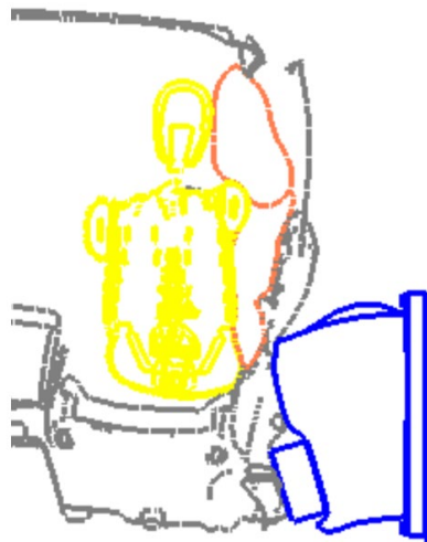
Figure 45. Deformation-based metrics (a) MDB deformation; (b) IIHS structural criteria and exterior vehicle crush
