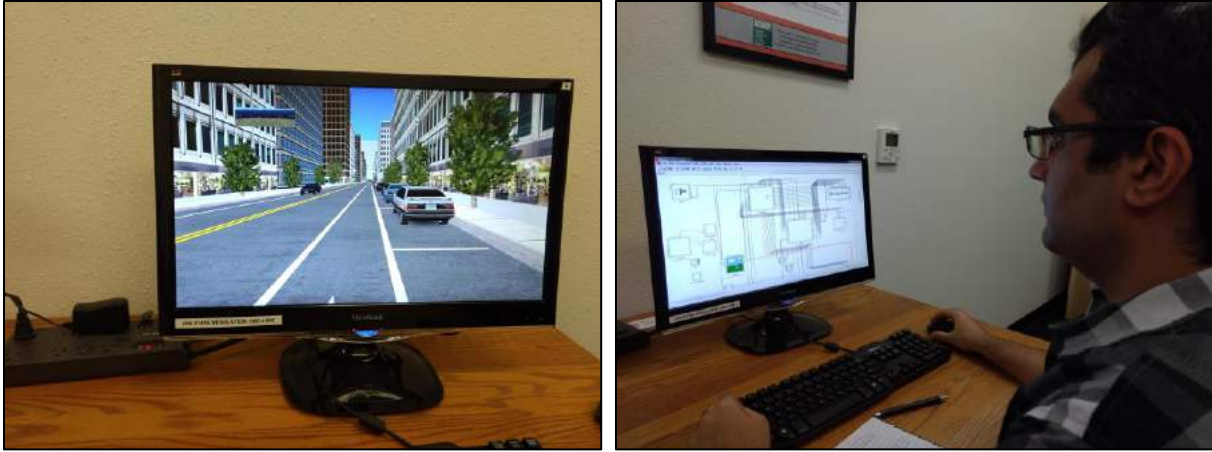
Figure 3.2 Operator workstation for the bicycling simulator. Left: Real-time monitoring of the simulated environment. Right: A researcher designing an experiment in SimCreator
