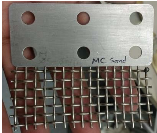
Figure 4.2 One example of a sieve and diffuser set inserted into the pluviator.
