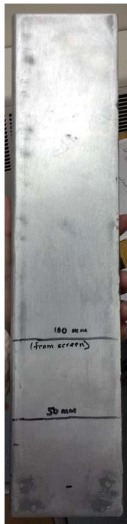
Figure 4.1 Rectangular pluviator for the preparation of cohesionless specimens.
