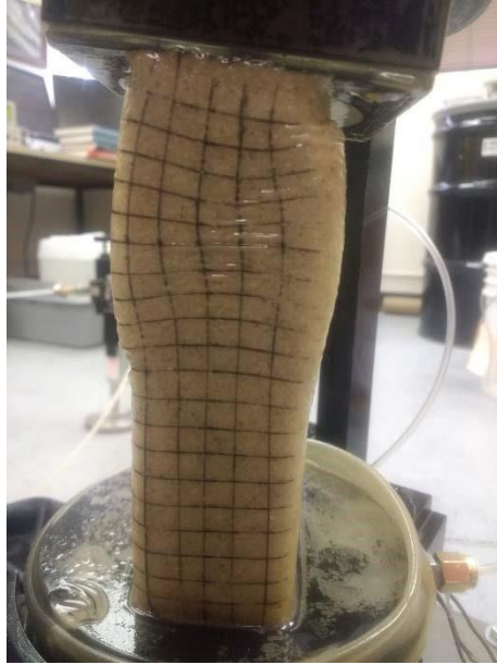
Figure 5.8 Test S-2 post-shear looking in the direction of no strain with two shear bands
