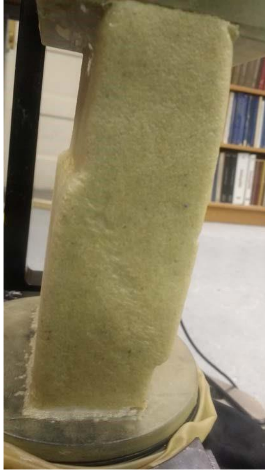
Figure 5.1 Shear band from end of test V-1
