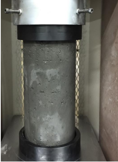
Figure 3.8 Compressive strength test
