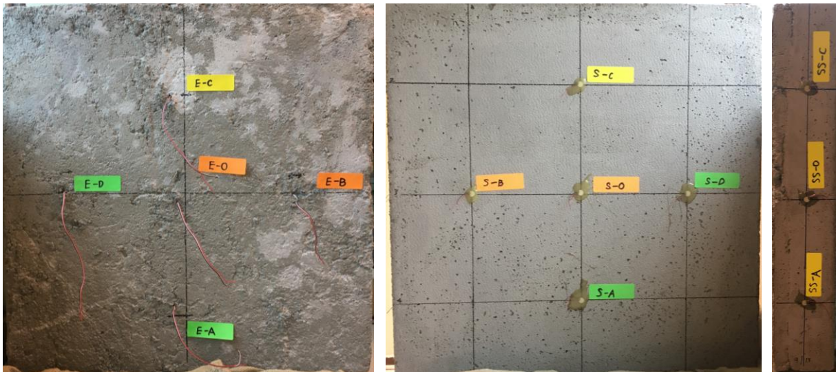
Figure 3.6 Labelled PZT patches on and embedded PZT cement modules in the concrete panel: embedded PZT cement modules (E-A to E-D and E-O), surface-mounted PZTs (S-A to S-D and S-O), and side surface-mounted (SS-A, SS-C and SS-O)
