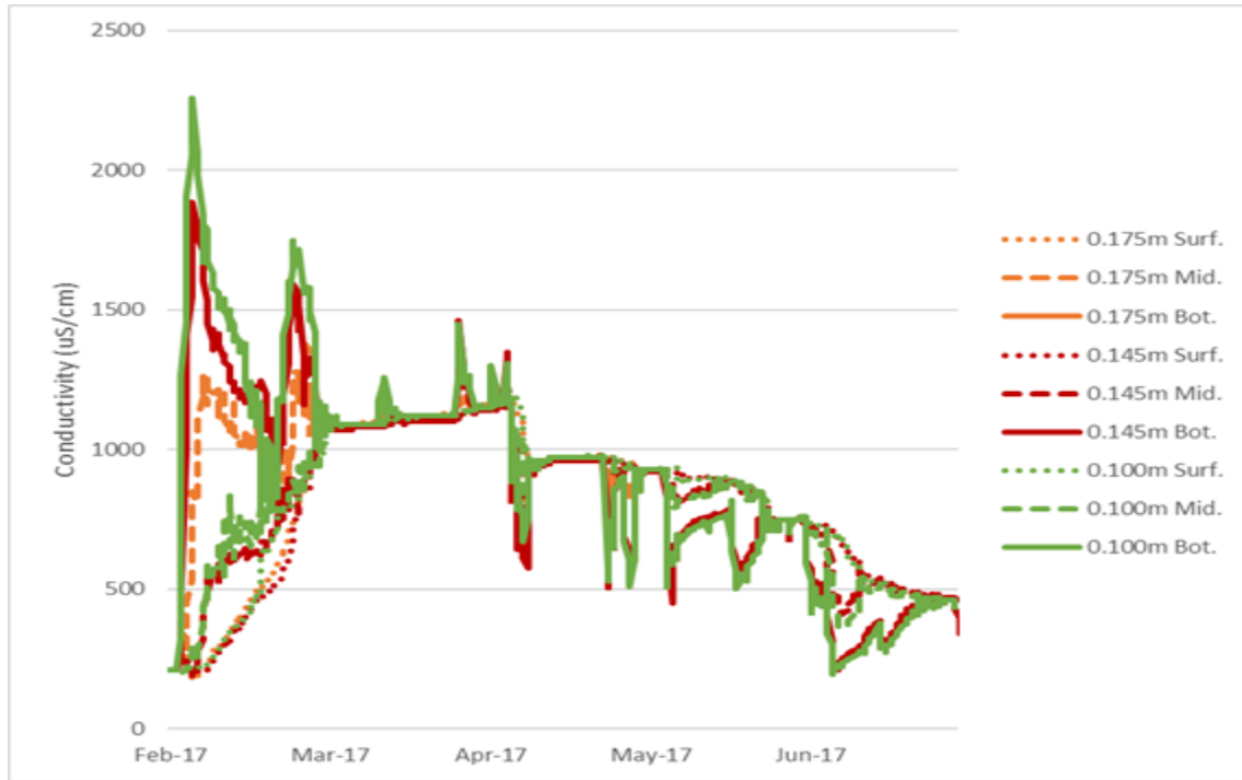
Figure 6: Comparison of electrical conductivity measurements at various depths (surface, middle, and bottom of the water column) and influence of modifying vertical grid resolution.
