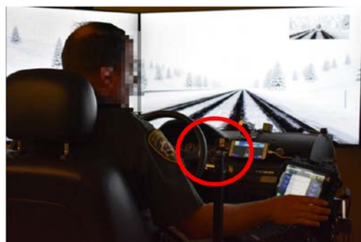
B- Subfigure B -HMI Mounting Location on the Driving Simulator for Highway Patrol
