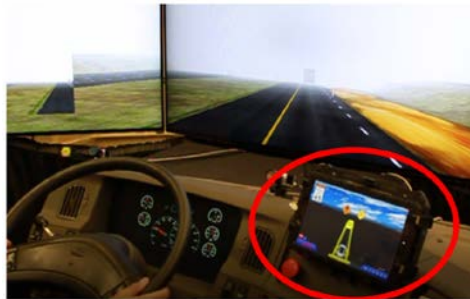
A- Subfigure A - HMI Mounting Location on the Driving Simulator for Truck Driver
