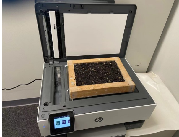
Figure 13. Apparatus used to Scan RAP for Grayscale-based Image Analysis
