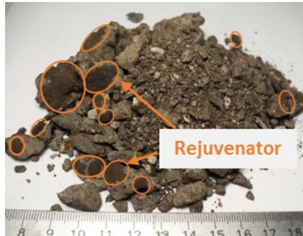
Figure 1. Non-uniform Dispersion of Rejuvenator in RAP when Added using the Traditional RAP Pretreatment Method (Xie et al., 2020)
