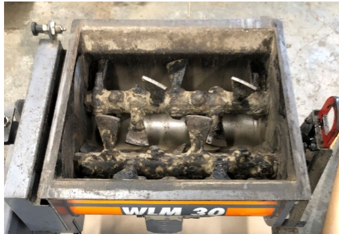
Figure 11. The Wirtgen Pugmill used to Pretreat RAP with Rejuvenators
