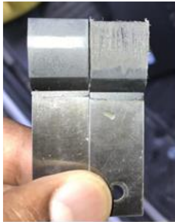
Figure 21 – Picture. Comparison of a new DFT rubber pad with the worn out DFT rubber pad after four measurements on calcined bauxite HFST.
