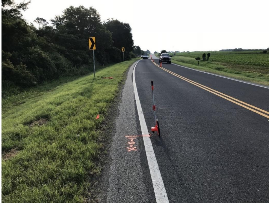
Figure 19 – Picture. Identification of spots in the middle of the curve site using a measuring wheel and a marking on the shoulder indicating the spot to collect data, I - Left wheel path, O - Right wheel path, X - non-wheel path.
