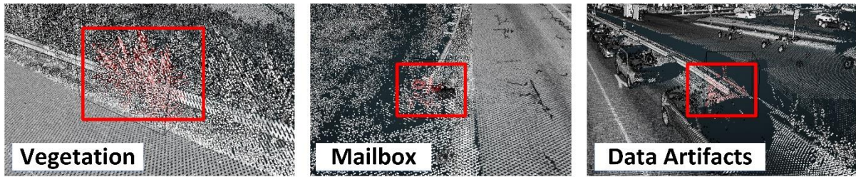
Figure 2.19: Misidentified damaged or missing terminals
