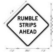
Figure C-46. Standard detail of temporary transverse rumble strips from Oregon DOT
