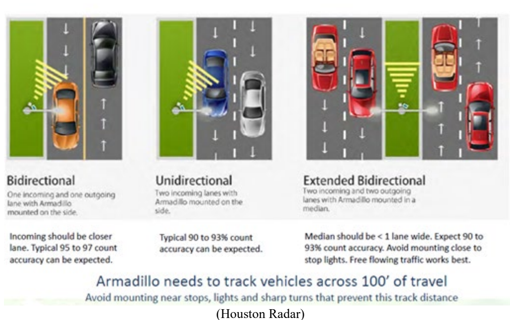
Figure 1. Tracker mounting options for Armadillo (Houston Radar)
