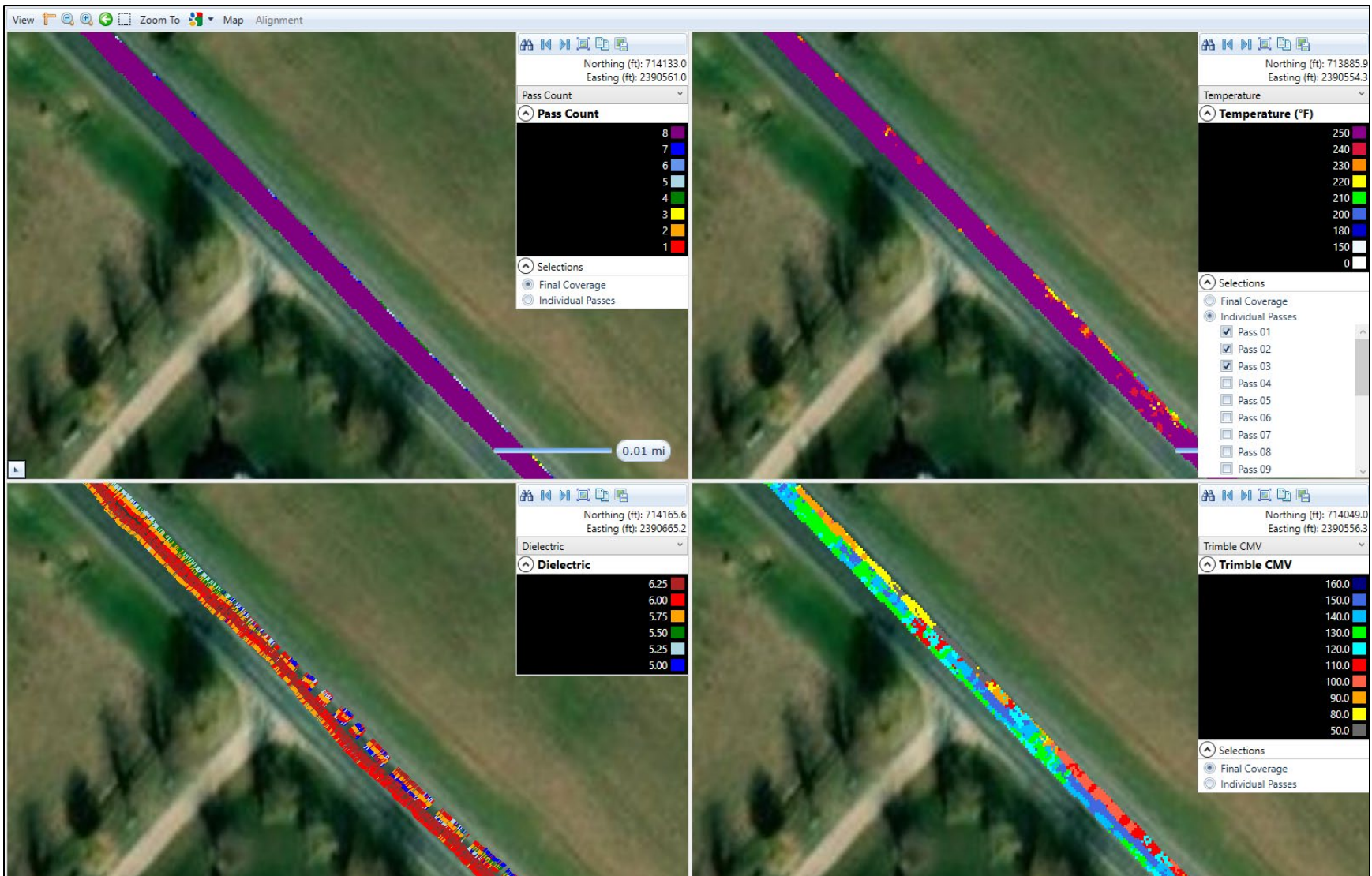
Figure 14. Screenshot. IC pass count (top left), IC temperature (top right), DPS (lower left), and IC ICMV (lower right) data.
