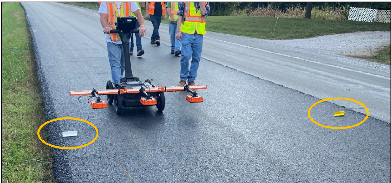
Figure 6. Photo. Temporary lane markings on either side of the pavement interfere with RDM readings (false low density, out of range density).
