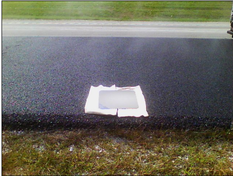
Figure 24. Photo. Improved reference object met the dimensions required and stayed below 150°F during testing.
