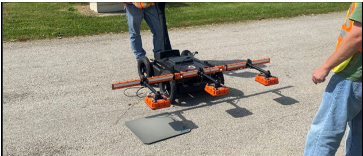
Figure 2. Photo. RDM 2.0 metal plate calibration.
