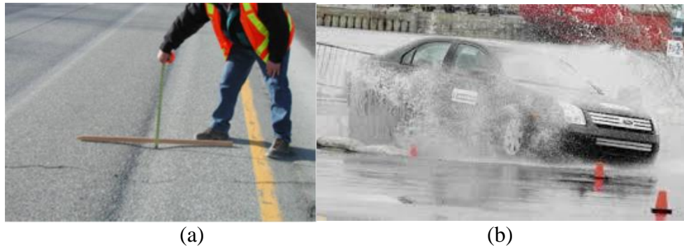
Figure 1.1 (a) Studded tire wear (after WSDOT) and (b) related hydroplaning.
