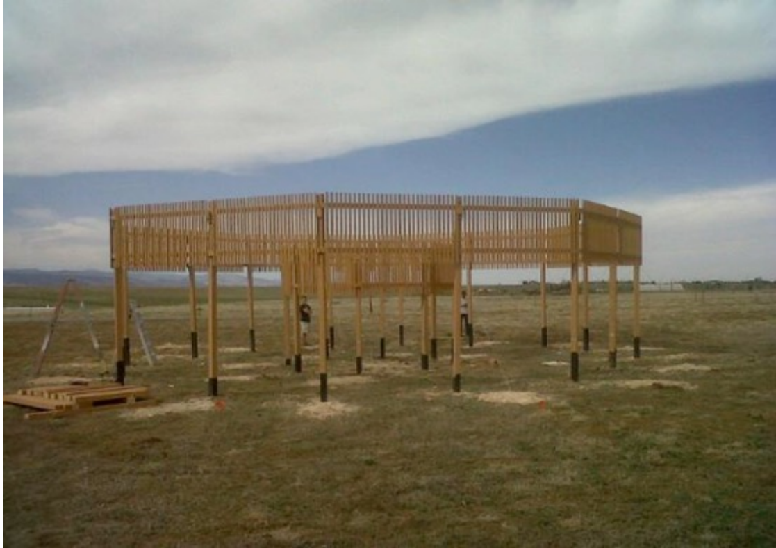
Figure 5. DFIR wind shield at the NCAR Marshall Field test site
