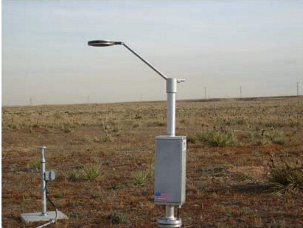
Figure 2. Hotplate TPS-3100 Total Precipitation Sensor
