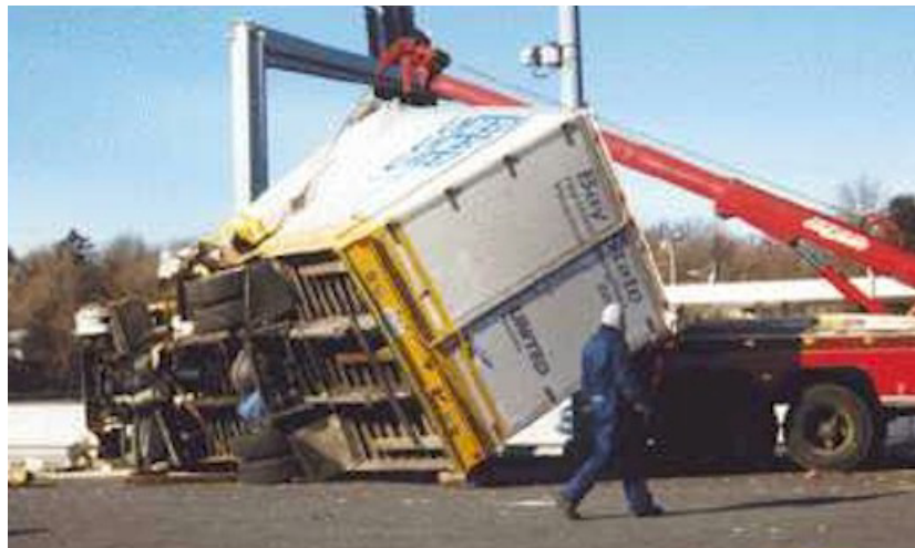
Figure 5. Use of a Heavy Crane Clearing a Major Incident (3)
