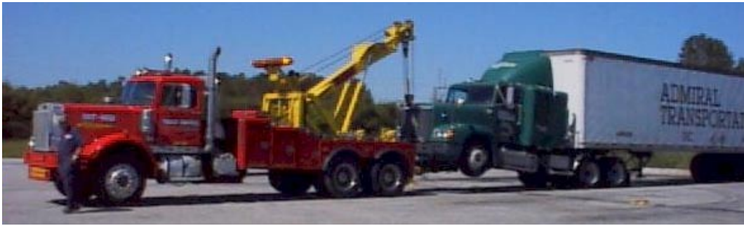
Figure 4. Use of a Heavy Tow Truck Clearing a Major Incident (3)
