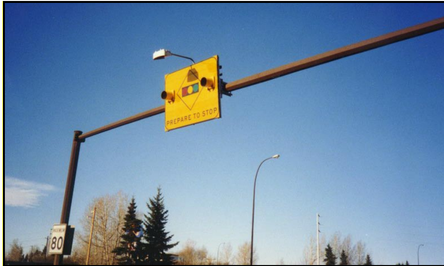
Figure 3. Advance Warning Flasher, Calgary, Alberta (13)
