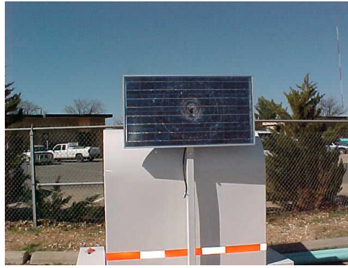
Figure 10. Vandalized Speed Trailer
