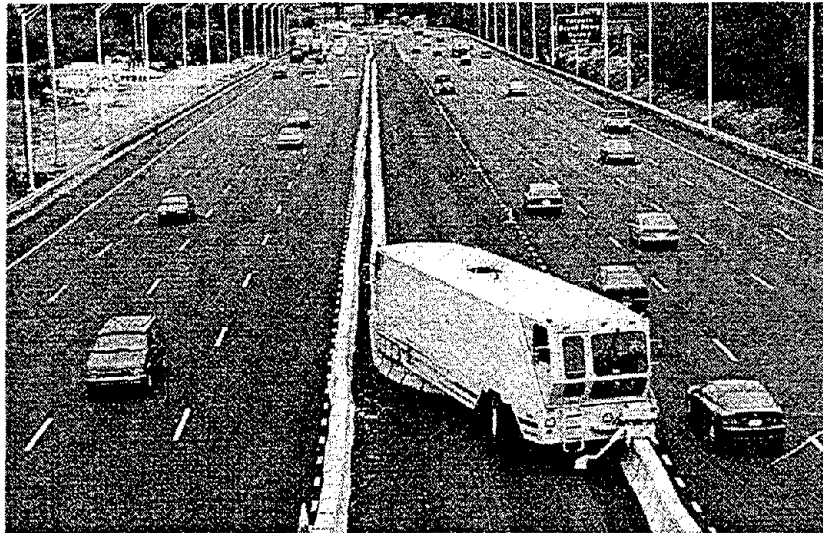
Figure 4. Reversal of a Contraflow HOV Lane Using a Barrier Transfer Machine (4).
