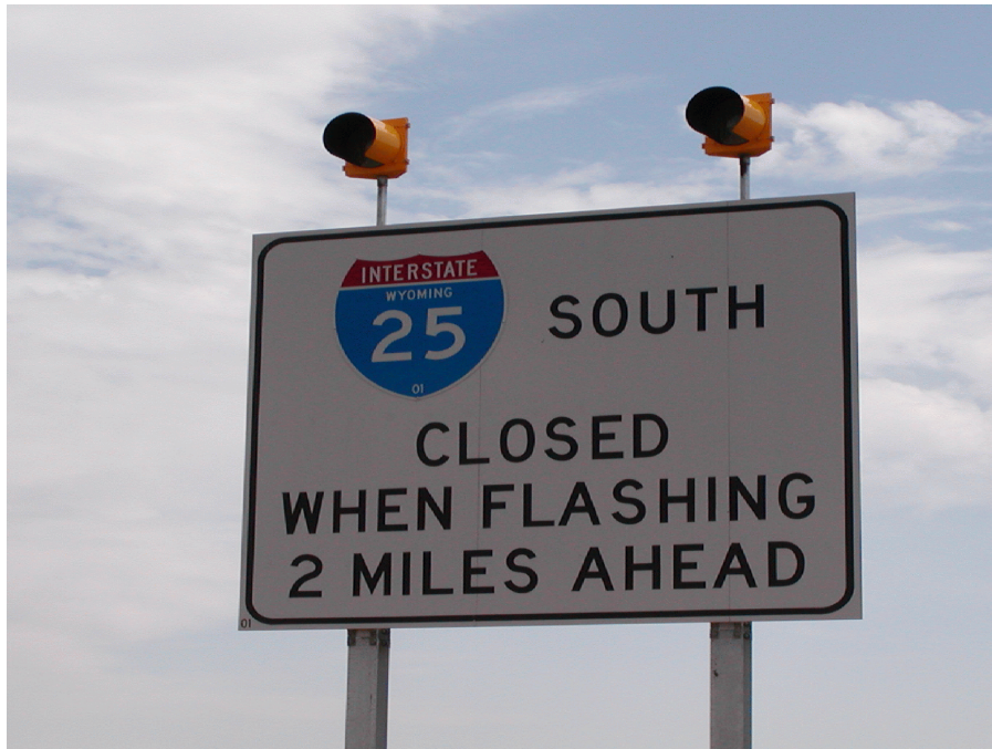
Figure 5. Sign with Flashing Beacons
