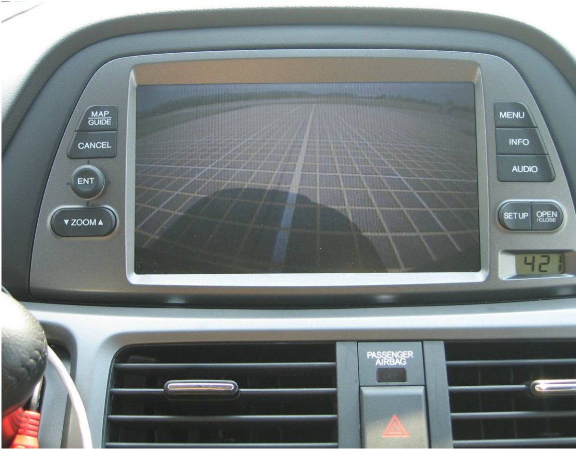
Figure 3. Rearview Video System Visual Display of the 2007 Honda Odyssey
