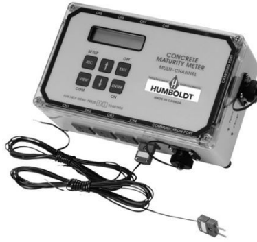
Figure 11. Maturity test apparatus with thermocouple (Helal et al. , 2015b)
