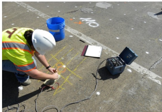
Figure 18. Corrosion Rate Test
