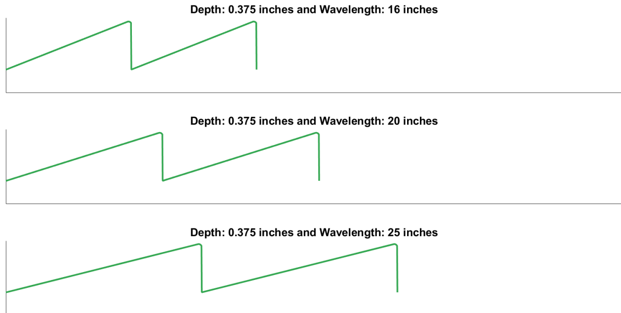
Figure 5.1: Side profiles of the sawtooth-long-climb-quick-drop design.
