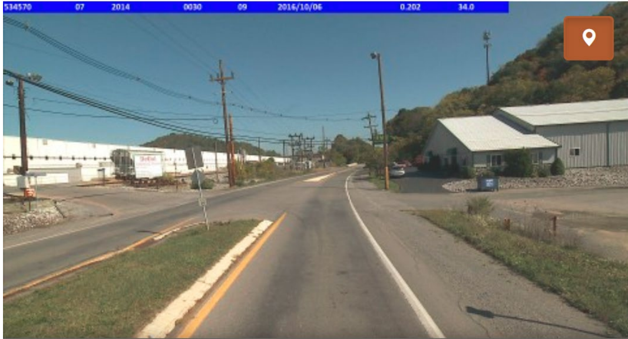
Figure 13. Example of access driveways to obtain access density (County 7, Route 2004, Segment 10)
