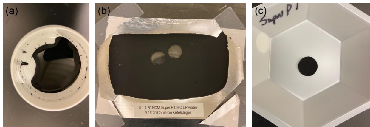
Figure 6. (a) Electrode slurry containing Super P ® carbon in Thinky Mixer Containers. (b) Picture after the slurry was casted on an aluminum current collector and dried. (c) Picture of electrode punched for coin-cell manufacturing.
