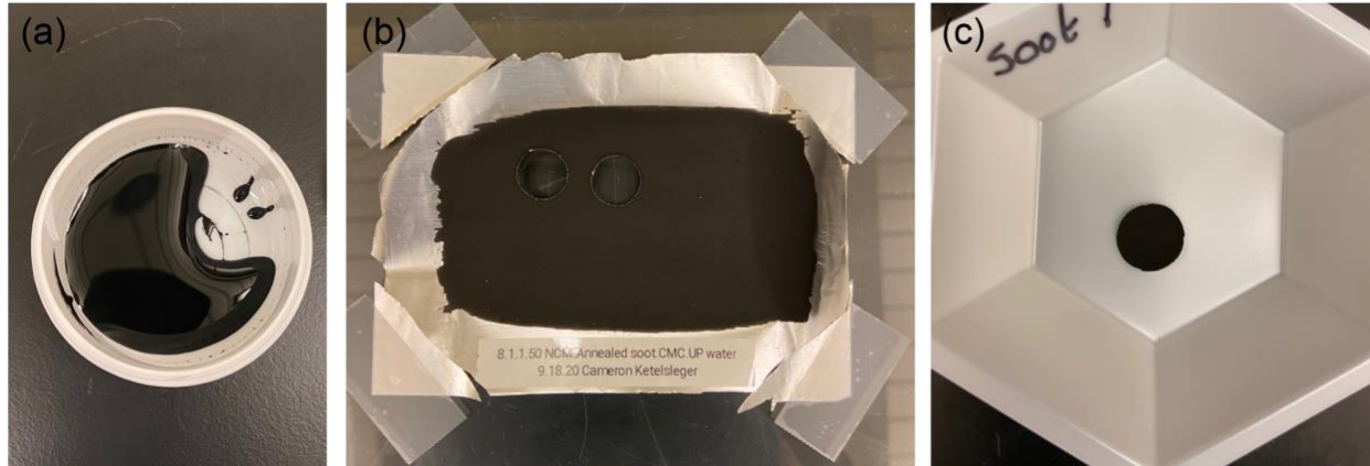
Figure 5. (a) Electrode slurry containing annealed diesel soot particles in Thinky Mixer Containers. (b) Picture after the slurry was casted on an aluminum current collector and dried. (c) Picture of electrode punched for coin-cell manufacturing.
