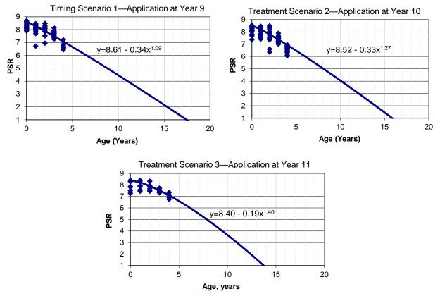
Figure 16. Post-treatment performance curves for the three mill-and-thin HMA overlay timing scenarios.
