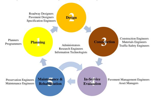
Figure 17. Five basic phases in the highway life cycle (modified from Zhang et al. 2003).
