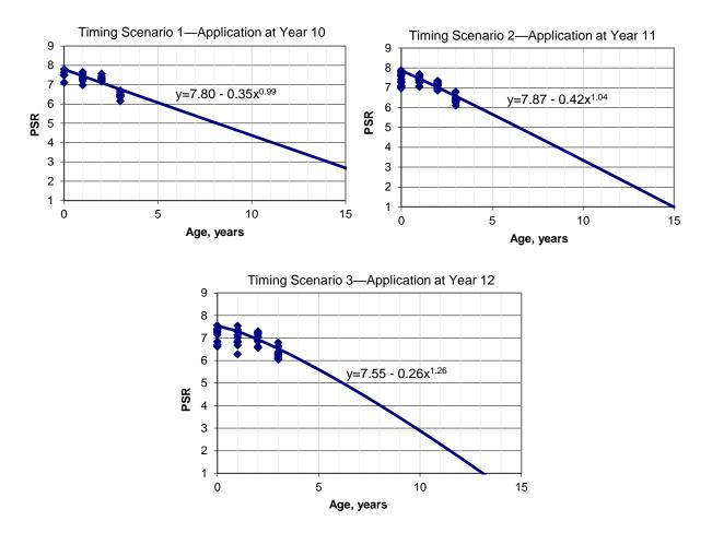
Figure 14. Post-treatment performance curves for the three chip seal timing scenarios.
