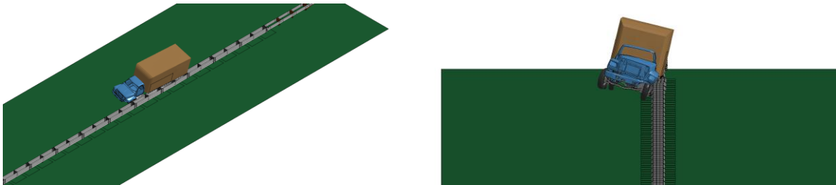
Fig. 4.66: Simulations of single-unit truck impacting the double-faced 29-inch steel-blockout Thrie-beam guardrail at 56 mph (90 km/h) and 15°.
