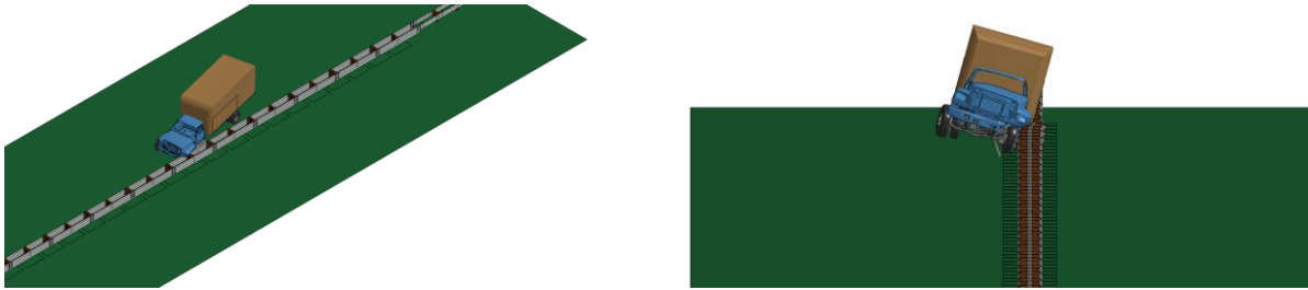
Fig. 4.65: Simulations of single-unit truck impacting the double-faced 29-inch wood-blockout Thrie-beam guardrail at 56 mph (90 km/h) and 15°.
