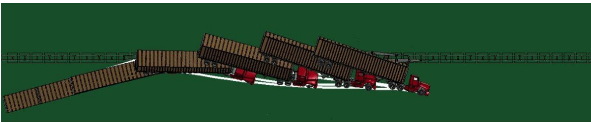
Fig. 4.69: A tractor-trailer impacting the double-faced 29-inch wood-blockout Thrie-beam guardrail at 50 mph (80 km/h) and 15°.
