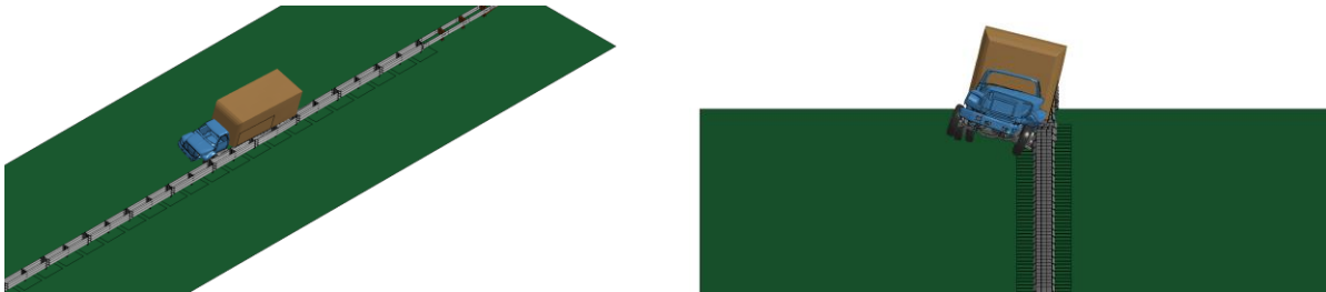
Fig. 4.103: Simulations of single-unit truck impacting the double-faced 31-inch steel-blockout Thrie-beam guardrail at 56 mph (90 km/h) and 15°.
