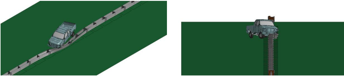
Fig. 4.57: Simulations of Ford F250 impacting the double-faced 29-inch steel-blockout Thrie-beam guardrail at 62 mph (100 km/h) and 25°.
