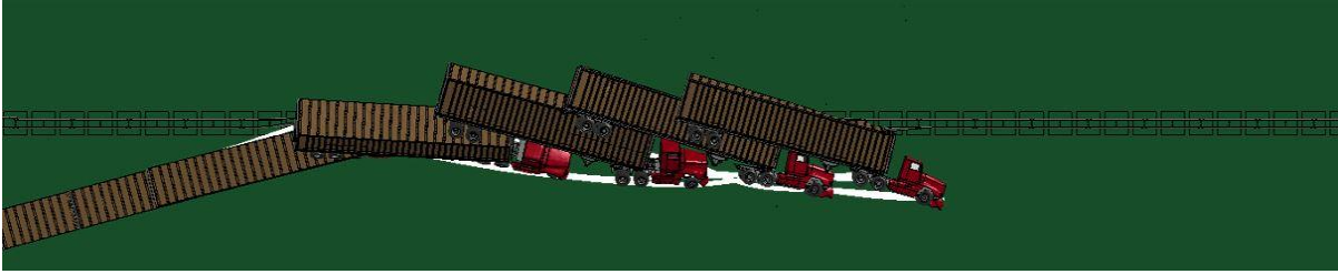
Fig. 4.107: A tractor-trailer impacting the double-faced 31-inch steel-blockout Thrie-beam guardrail at 50 mph (80 km/h) and 15°.
