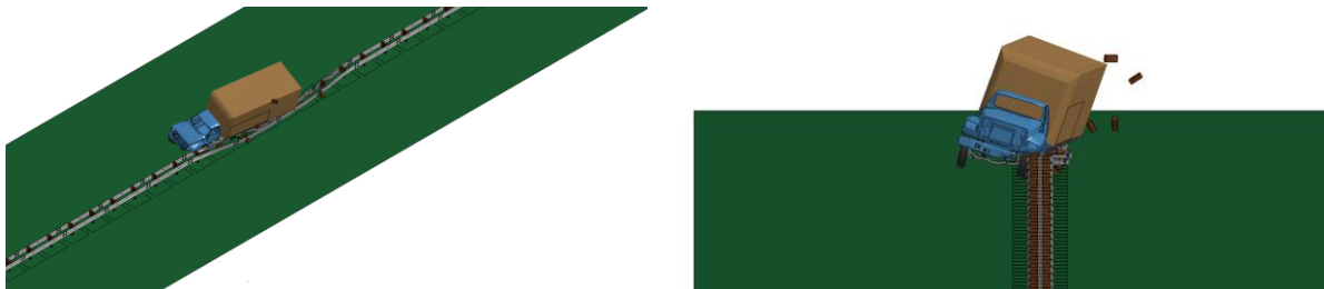
Fig. 4.35: Simulations of a single-unit truck impacting the double-faced 31-inch W-beam guardrail at 56 mph (90 km/h) and 15°.
