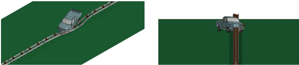
Fig. 4.30: Simulations of Ford F250 impacting the double-faced 31-inch W-beam guardrail at 62 mph (100 km/h) and 25°.
