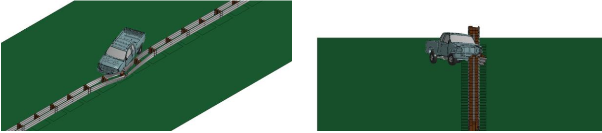
Fig. 4.56: Simulations of Ford F250 impacting the double-faced 29-inch wood-blockout Thrie-beam guardrail at 62 mph (100 km/h) and 25°.
