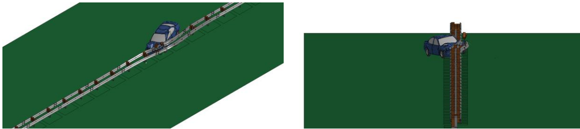
Fig. 4.25: Simulations of Dodge Neon impacting the double-faced 31-inch W-beam guardrail at 62 mph (100 km/h) and 25°.
