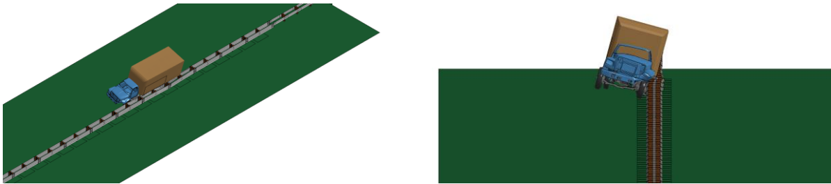
Fig. 4.102: Simulations of single-unit truck impacting the double-faced 31-inch wood-blockout Thrie-beam guardrail at 56 mph (90 km/h) and 15°.
