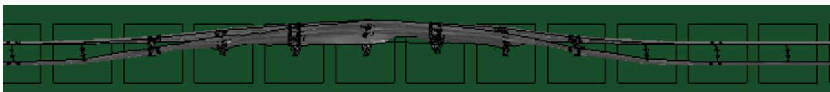
Fig. 4.111: Maximum dynamic deflection of the double-faced 31-inch steel-blockout Thrie-beam guardrail at 50 mph (80 km/h) and 15° and impacted by a tractor-trailer.
