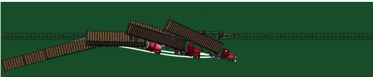
Fig. 4.106: A tractor-trailer impacting the double-faced 31-inch wood-blockout Thrie-beam guardrail at 50 mph (80 km/h) and 15°.
