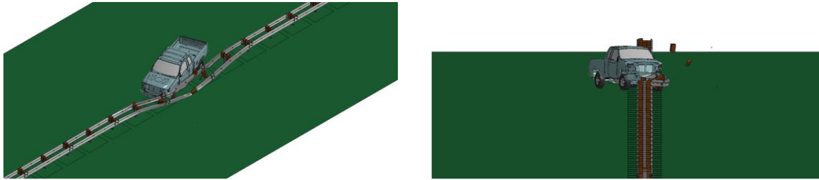
Fig. 4.10: Simulations of Ford F250 impacting the double-faced 29-inch W-beam guardrail at 62 mph (100 km/h) and 25°.
