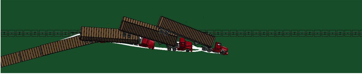
Fig. 4.70: A tractor-trailer impacting the double-faced 29-inch steel-blockout Thrie-beam guardrail at 50 mph (80 km/h) and 15°.
