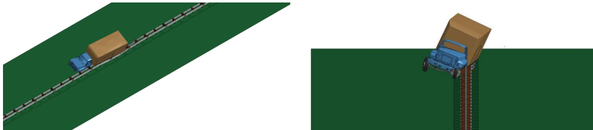
Fig. 4.15: Simulations of the single-unit truck impacting the double-faced 29-inch W-beam guardrail at 56 mph (90 km/h) and 15°.
