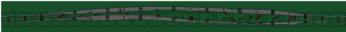
Fig. 4.110: Maximum dynamic deflection of the double-faced 31-inch wood-blockout Thrie-beam guardrail at 50 mph (80 km/h) and 15° and impacted by a tractor-trailer.
