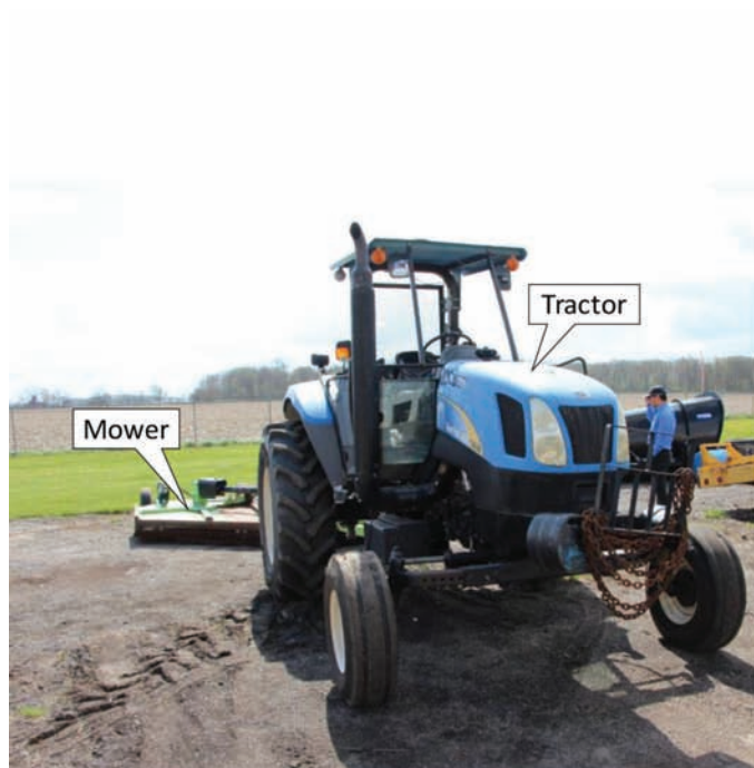
(a) Tractor with 15' flex-wing rotary mower
