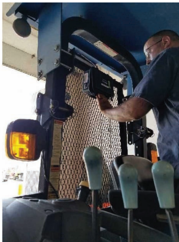
(b) Installation of GPS device on the mesh behind driver seat
