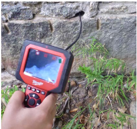
Figure 3-2: Demonstrating use of borescope to inspect crevice in bridge abutment
