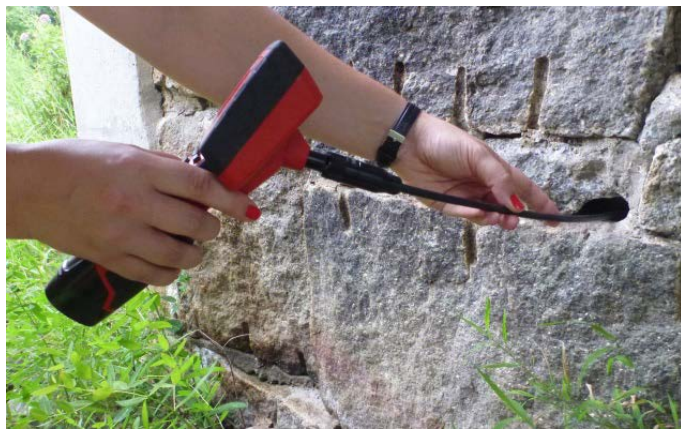
Figure 3-2: Demonstrating use of borescope to inspect crevice in bridge abutment
