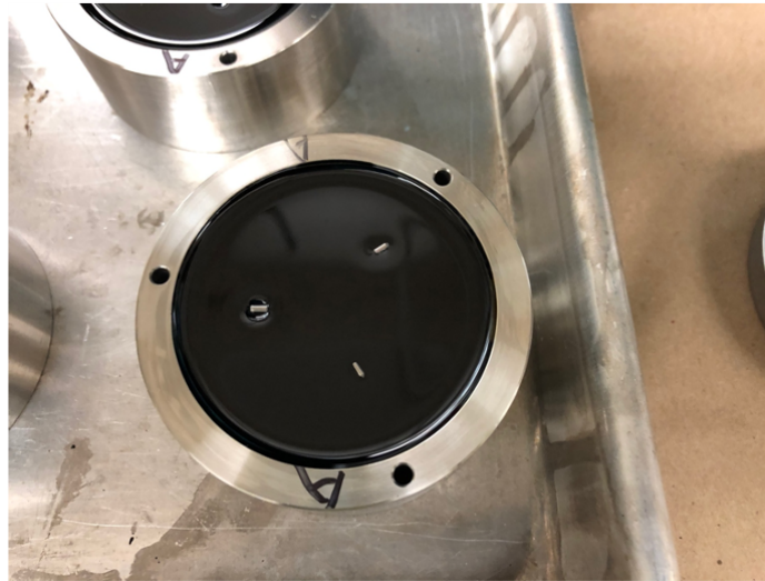
Figure A.4. Closer view of three dowels used for film thickness control placed on the liquid binder in the heated bottom plate of the poker chip assembly.
