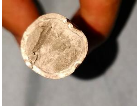
Metallic object found in grout
