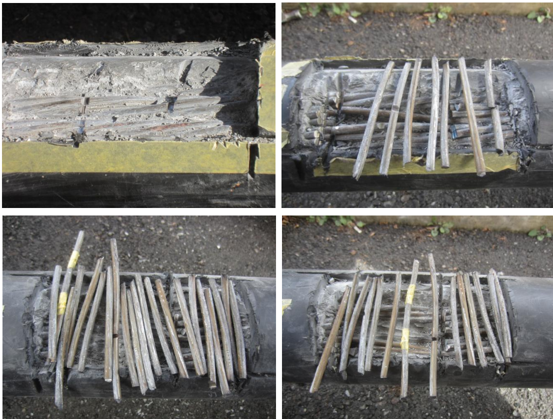
Figure 13. Removed wires for 0.6, 4.5, 9.1, and 13.6 percent section losses (clockwise from top left).
