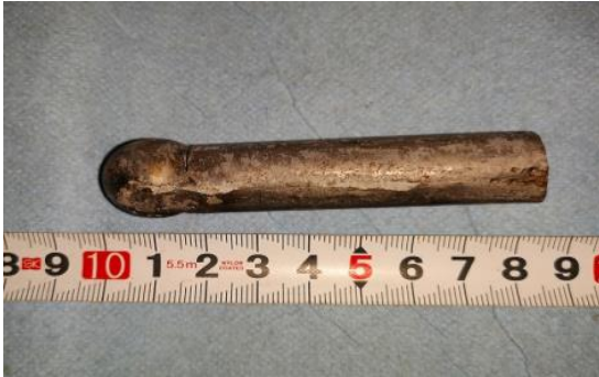
Metallic object found in grout
