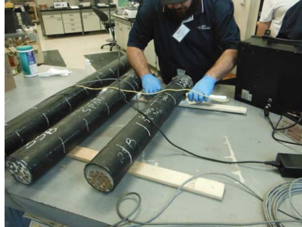
Photograph 5- Sonic/ultrasonic impact echo testing
