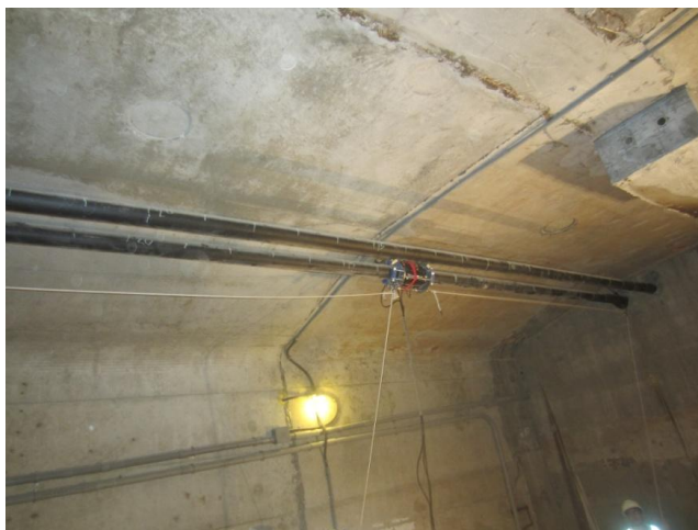
Figure 30. Magnetizer on a high elevation horizontal section.
