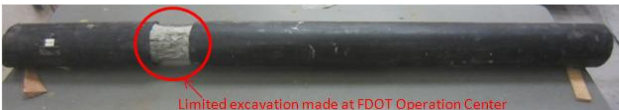
Figure 46. Tendon sample #2 before full autopsy.
