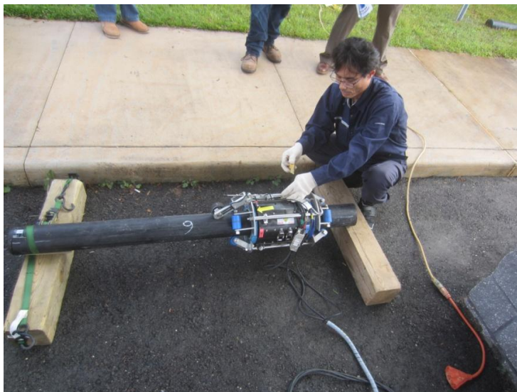
Figure 11. Calibration setup for tendon sample #1.
