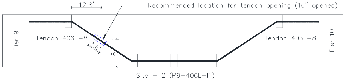
Figure 4-4: Tendon verification at site 2
