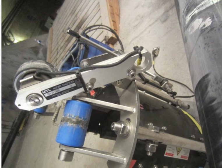
Figure 5. Rotary encoder type distance meter.
