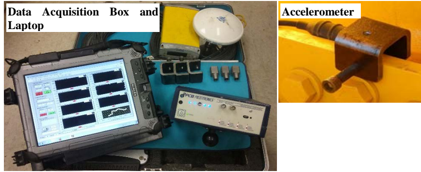
Figure 5.3 – Components of the Data Acquisition System Developed at UTEP.
