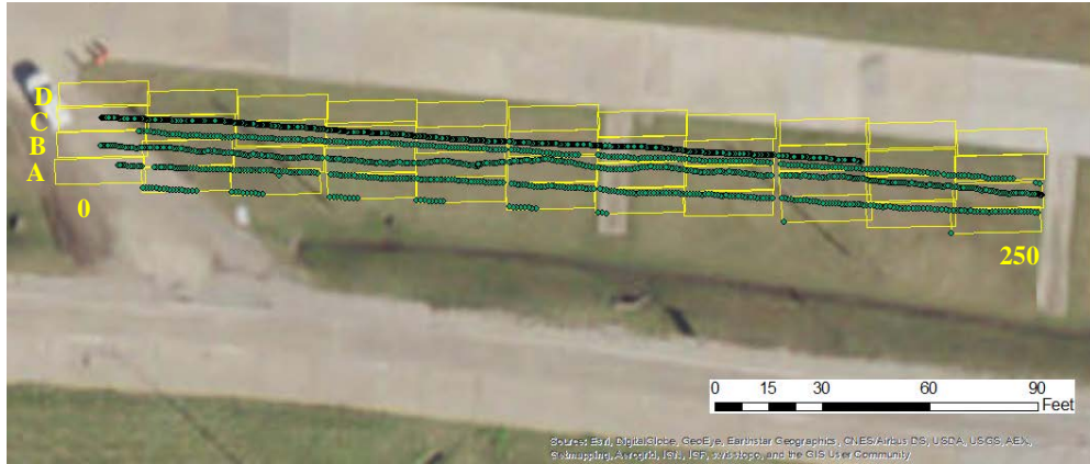
Figure H.13 – Data Collected by IC Roller on top of Base Divided in Rectangular Buffered Areas
