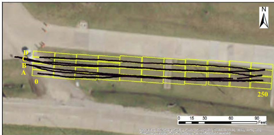
Figure H.6 – Data Collected by IC Roller on top of LTS Divided in Rectangular Buffered Areas.
