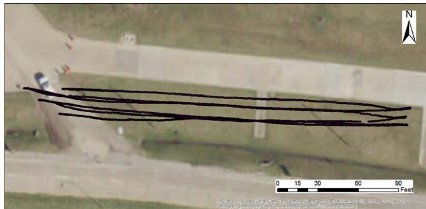
Figure H.4 – IC Data Points Collected During Proof-Mapping of Subgrade Layer
