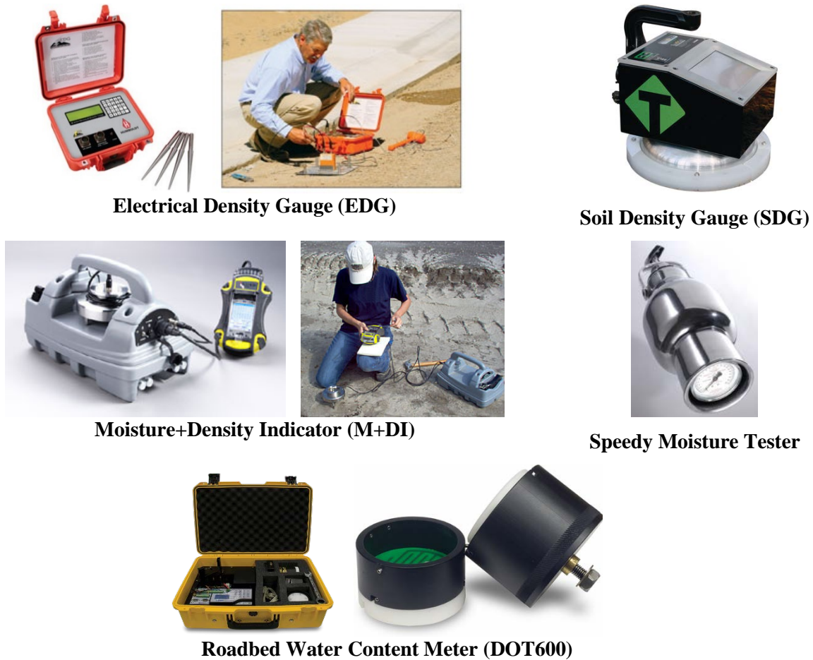
Figure 2.6 – Non-nuclear moisture and density measurement devices.
