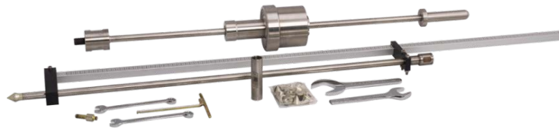
Figure 2.1 – Dynamic Cone Penetrometer (DCP).
