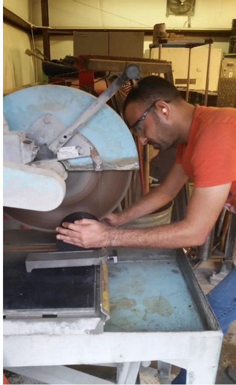
Figure 4.7: Trimming a bottom part of pavement core
