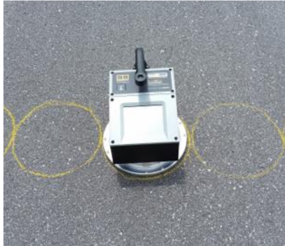
Figure 4.3: In-place, non-nuclear density gauge
