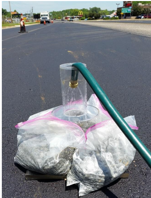
Figure 4.5: In-place pavement infiltration
