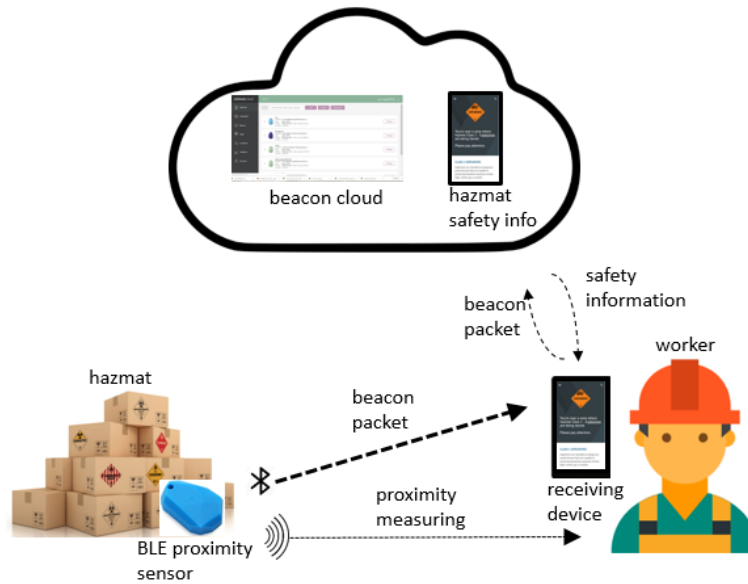
Figure 4.1 Schematic diagram of the BLE based feedback system
