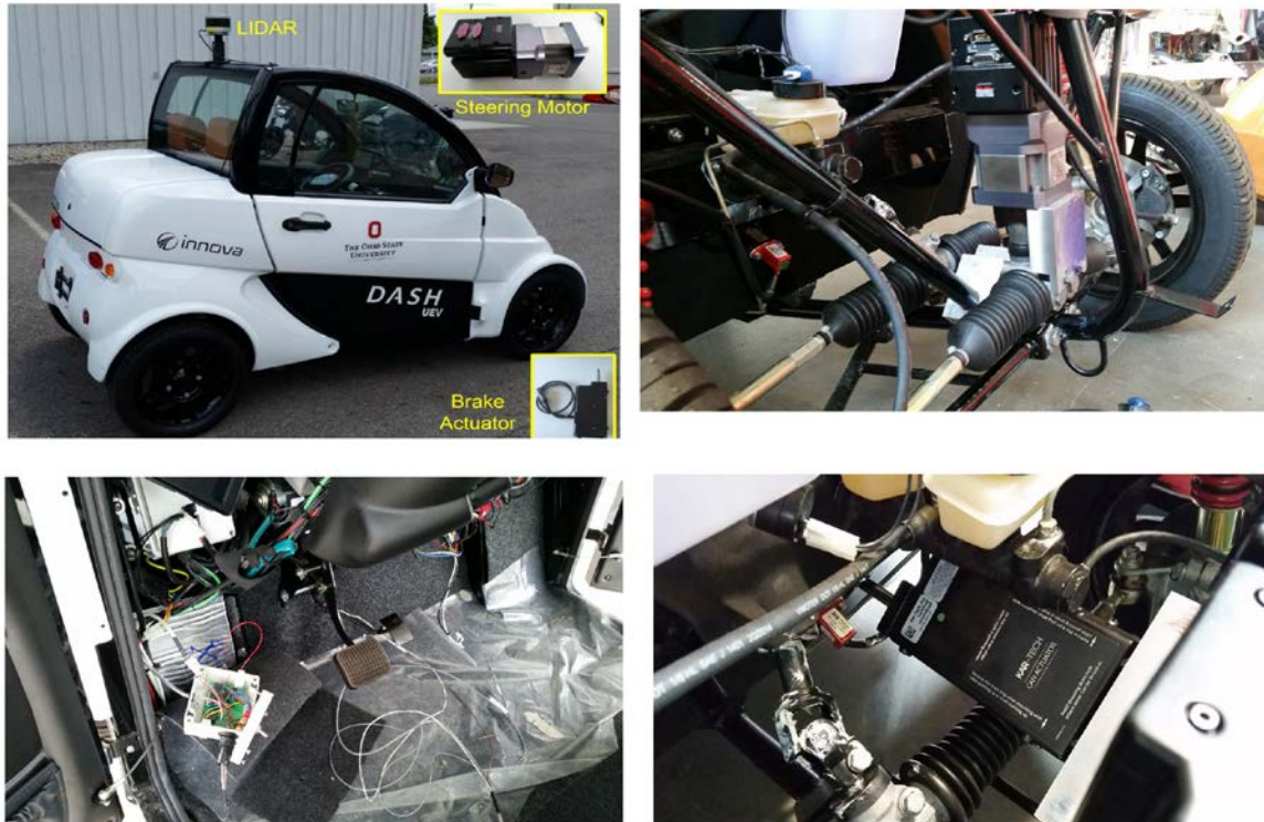
Figure 3. Dash EV drive-by-wire system.
