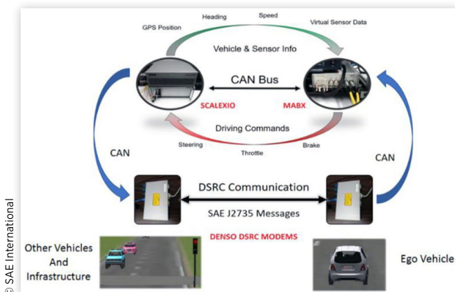
FIGURE 14 HiL equipment and communication.
