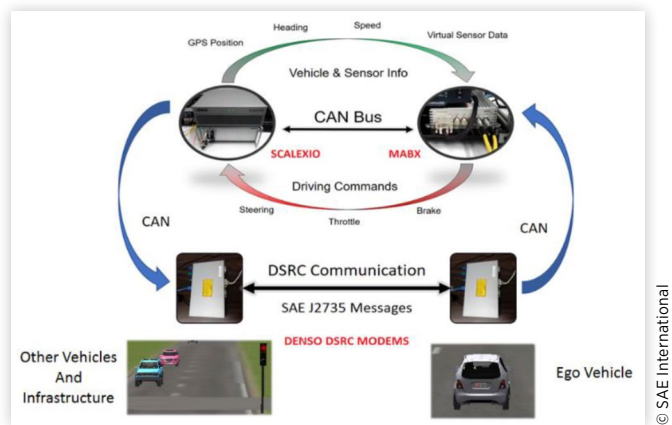
FIGURE 15 HiL equipment and communication.
