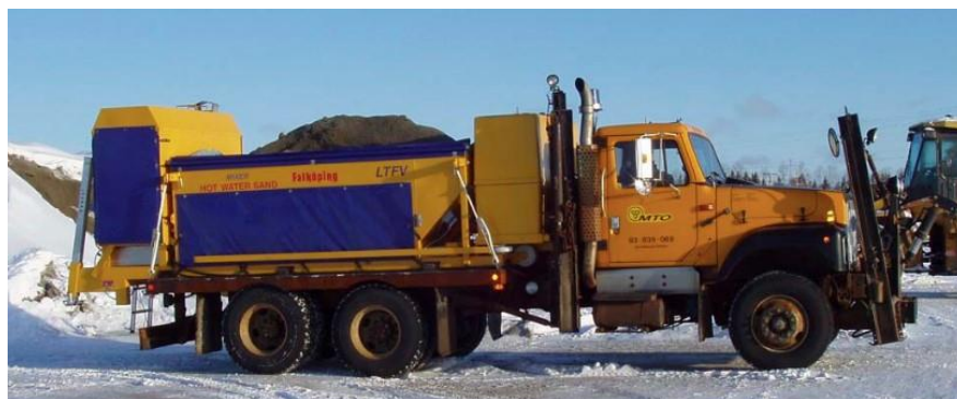
Figure 2.5. Hot water sander (Perchanok et al., 2010)
