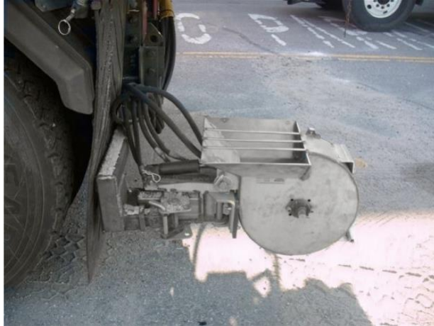
Figure 2.8. Zero-velocity spreader equipped on a truck (Thompson Engineering Company, 2014)
