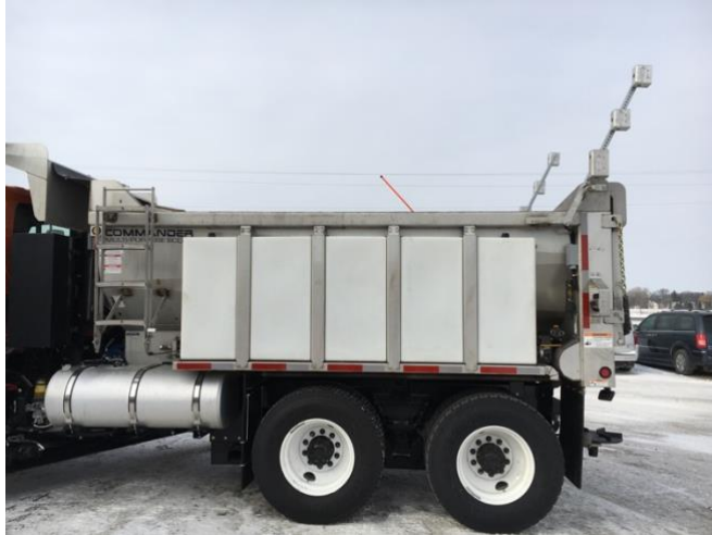
Figure 3.3. Tank with 400 gallons capacity (courtesy of North Dakota DOT)
