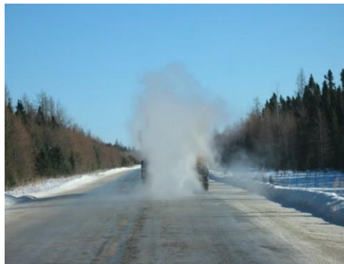
Figure 2.3. Fog cloud following the hot water sanding spreader (Perchanok et al., 2010)
