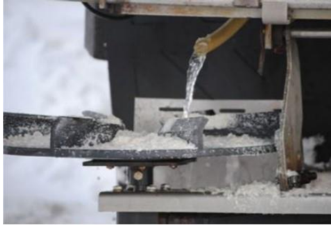
Figure 2.6. Basic on-board pre-wetting operation (Minnesota DOT)
