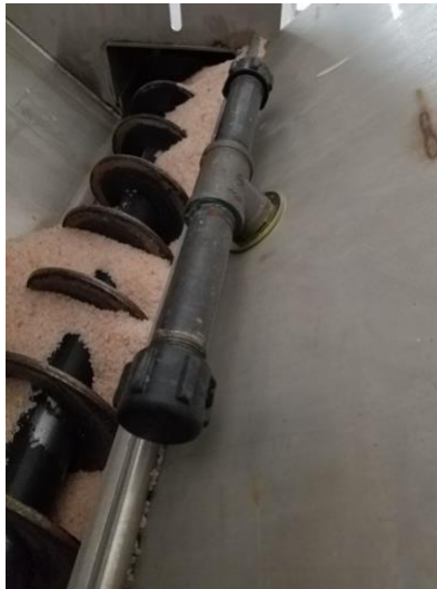
Figure 3.5. Auger trough with a pre-wetting delivery pipe (courtesy of North Dakota DOT)
