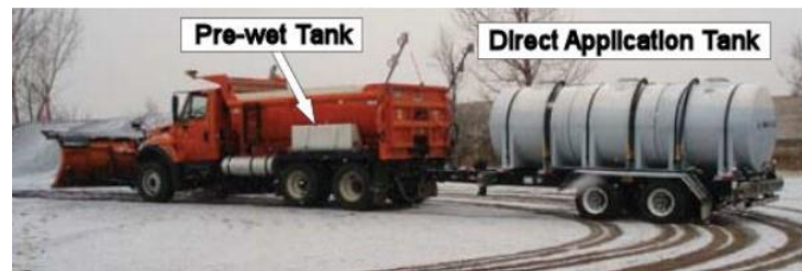
Figure 2.4. Hopper-side mount pre-wet tank and liquid tank for direct liquid application (North Dakota DOT)
