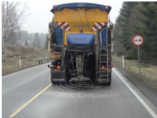
Figure 2.9. Spreading of pre-wetted fine graded salt in Norway (Hanke et al., 2019)
