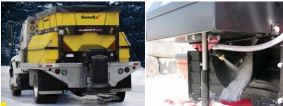
Snow Ex Super Maxx II 6 cubic yard spreader with integrated pre-wet system
