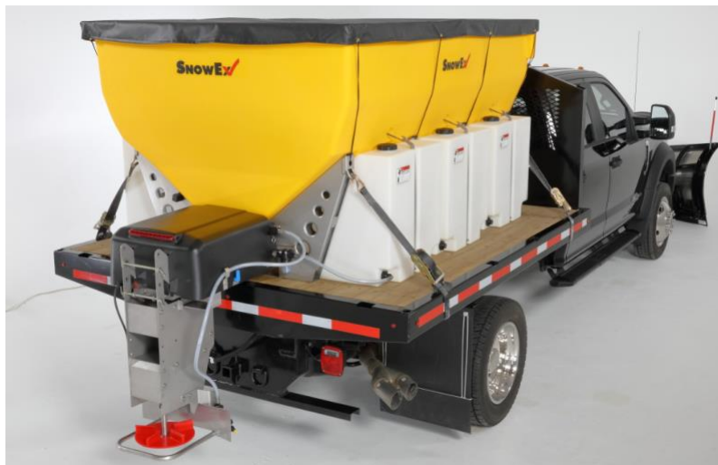
Figure 5.2. SnowEx tanks have been designed to fit in between the legs of the hopper as show in the photo above.
