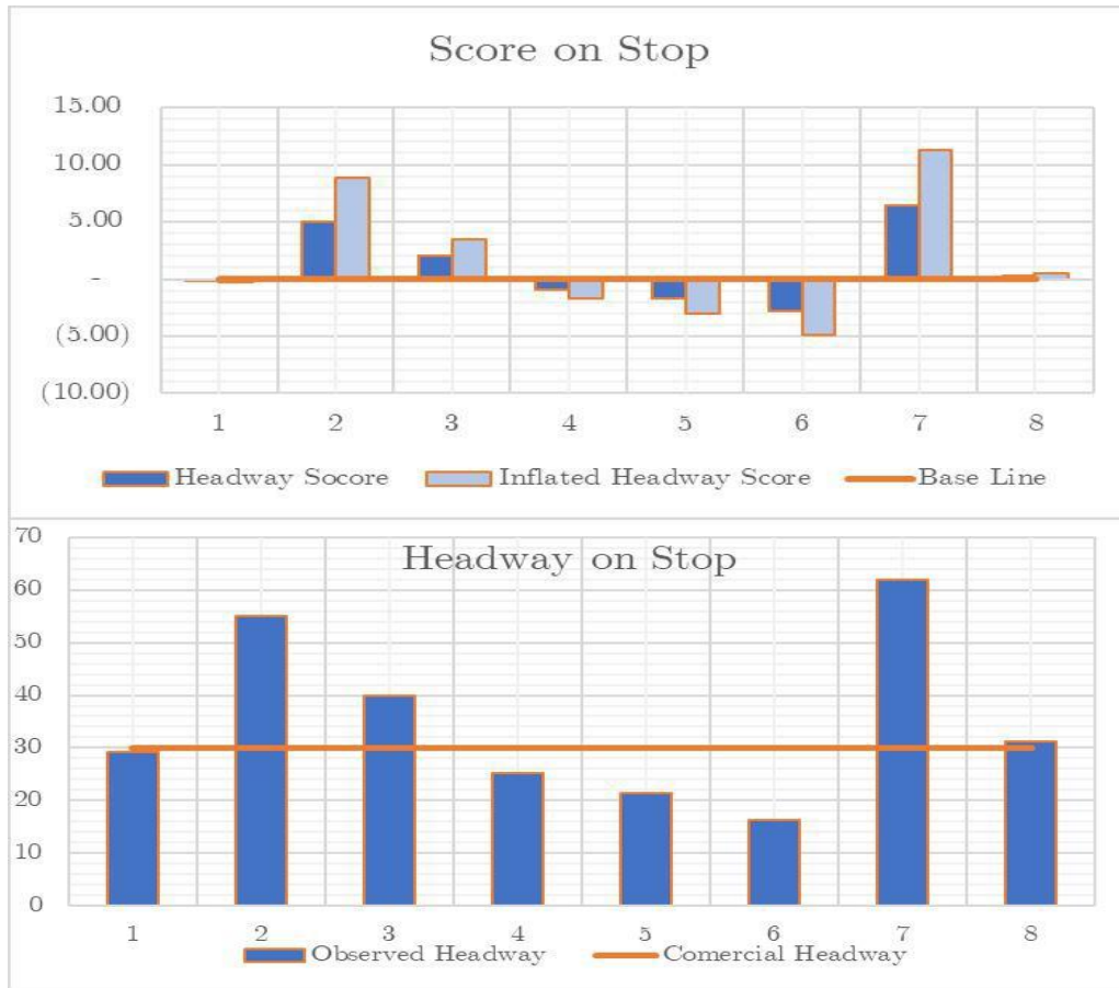
Figure 40 Comparison between the Observed Headway Measured at a Stop, the Commercial Headway and the Headway Affected by the Uniformity of Arrivals or Inflated Headway
