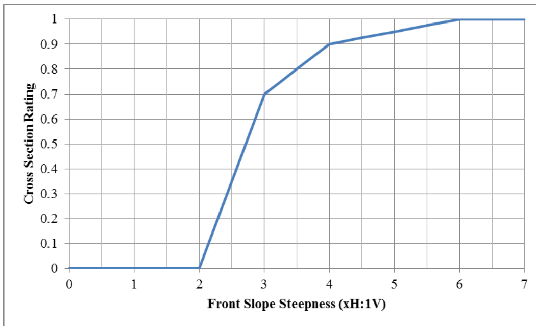
Figure 35. Front Slope Rating Curve.
