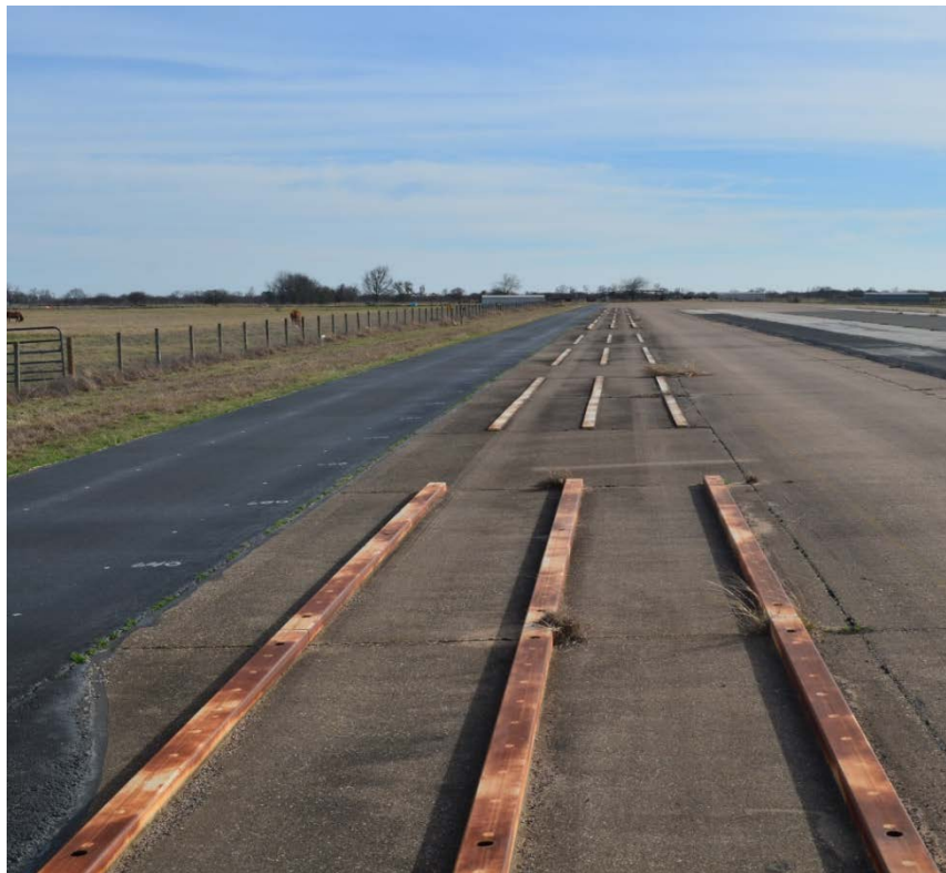
Figure 14. Rut Track Located at Texas A&M RELLIS Campus with Inverted Rut Plates of Known Dimensions.
