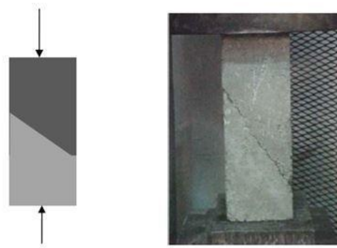
Figure 2: Slant Shear test format
