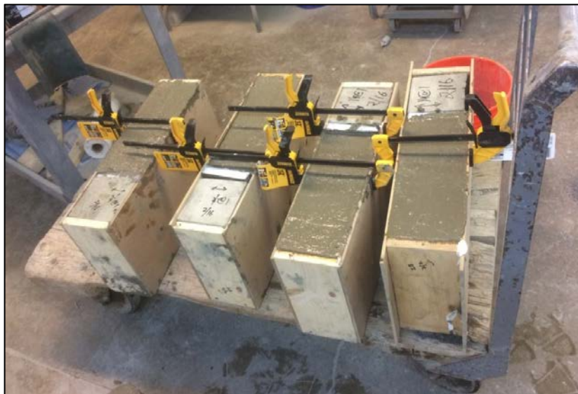
Figure 14: Composite specimen with freshly poured overlay concrete
