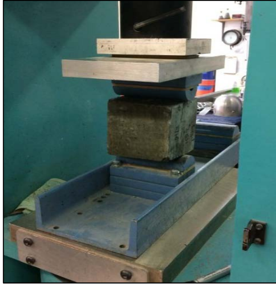
Figure 20: Testing of composite specimen for the Split-Prism test (Tensile Bond Strength)
