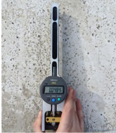
Figure 4-27: Measurement of "top" face of block using mechanical strain gauge with digital indicator of 0.0001" precision.
