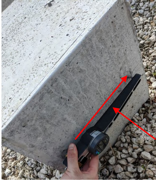
Figure 4-29: Measurement of "right" face of block with applied pressure in the direction of the red arrows.
