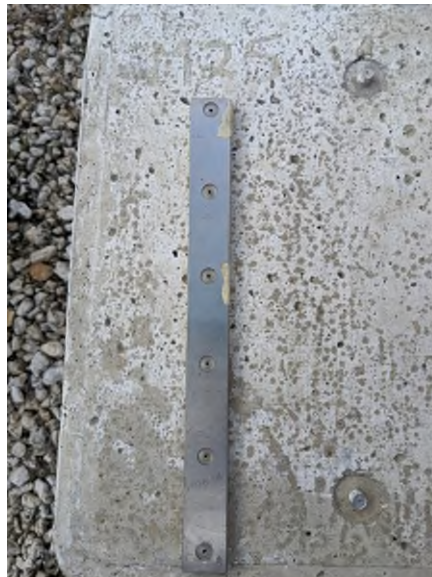
Figure 4-28: Reference bar used to calibrate the comparator before each measurement.
