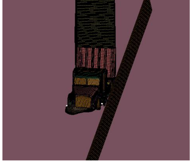
Figure 6.18 At t= 0.52 s, after Impact, No Contact with the Barrier
