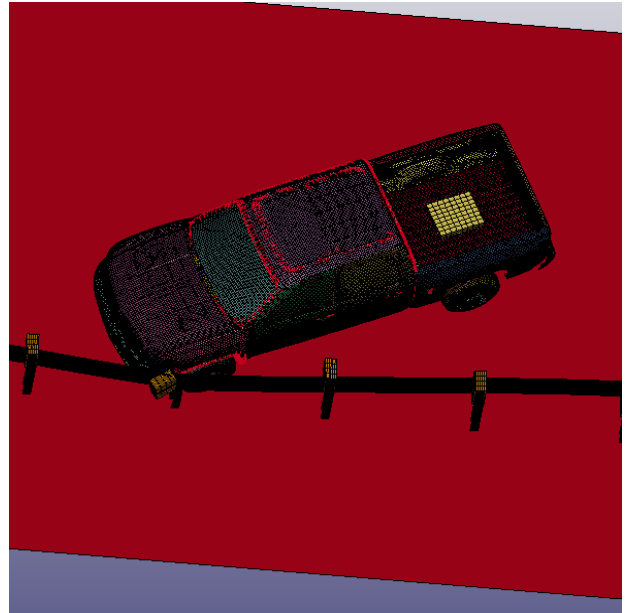
Figure 4.7 At t=0.05 s, the First Wooden Block Fails
