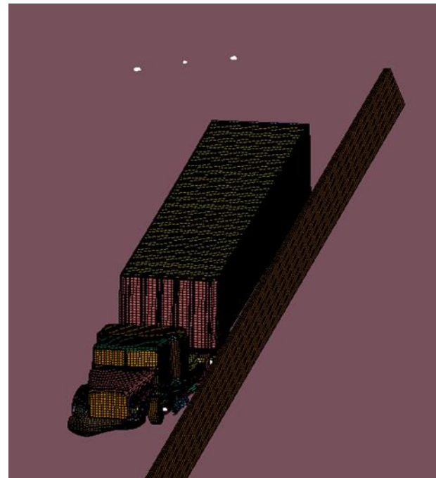
Figure 6.20 At t=0.83 s, Trailer Comes in Contact and Slides Along Barrier
