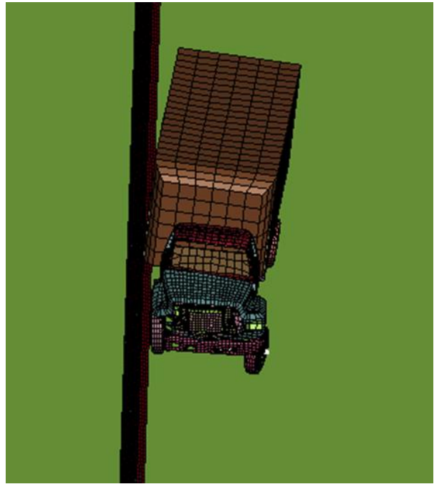
Figure 5.15 At t=0.32 s, the Back Tires Ride the Barrier and Slide against it
