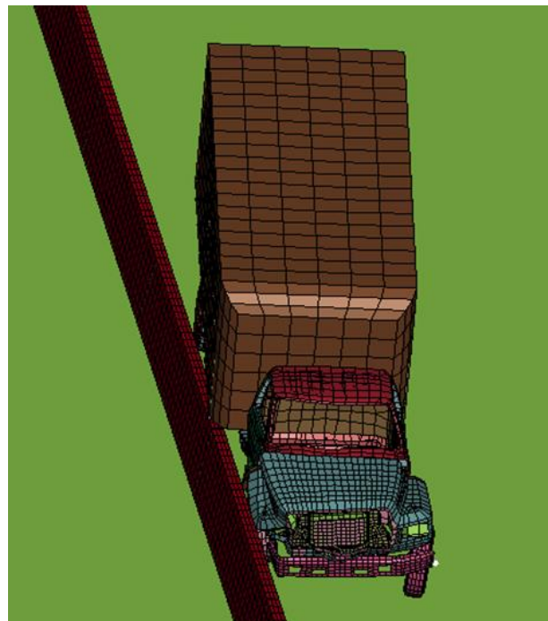
Figure 5.13 At t=0.2 s, the Trailer Overrides the Barrier
