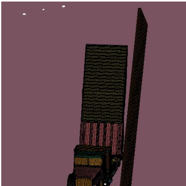
Figure 6.19 At t=0.75 s, Contact of Rear Part of Trailer with Barrier
