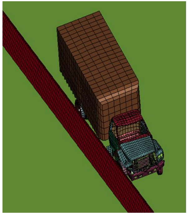
Figure 5.17 At t=0.65 s, Both Front and Back Tires Slide against the Barrier
