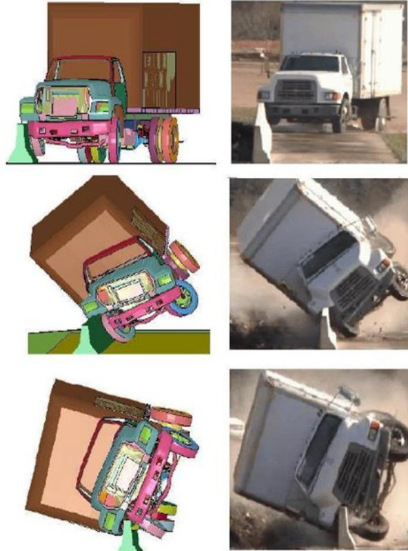
Figure 2.3 FEM vs Real Crash Test of an SUT (Esfahani, 2008)
