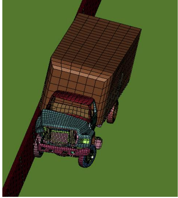
Figure 5.23 At t=1.31 s, the Truck is Diverted with Wheels Down
