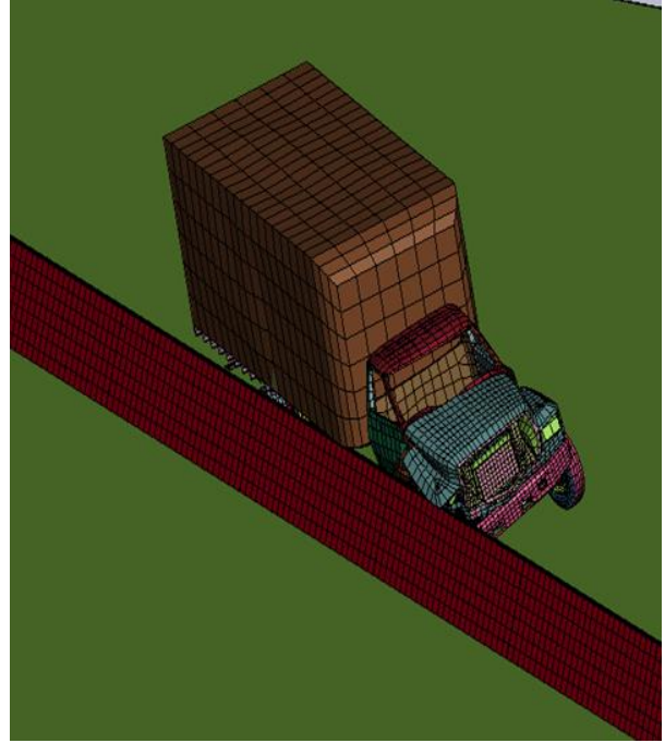
Figure 5.19 At t=0.81 s, the SUT Body Slides against the Barrier
