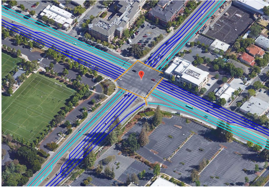
Figure 2.6 MAP message aerial view of Page Mill Rd. and El Camino Real in Mountain View, CA (California CV Testbed et al., 2020).
