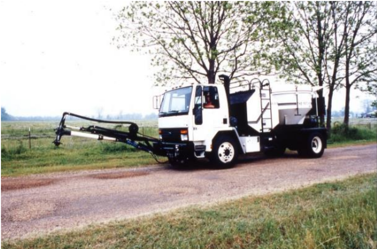
Figure 41. Spray Injection Patch Truck
