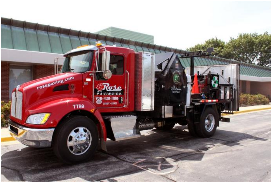
a. Heater Patching Truck (Rose Paving, 2013)
