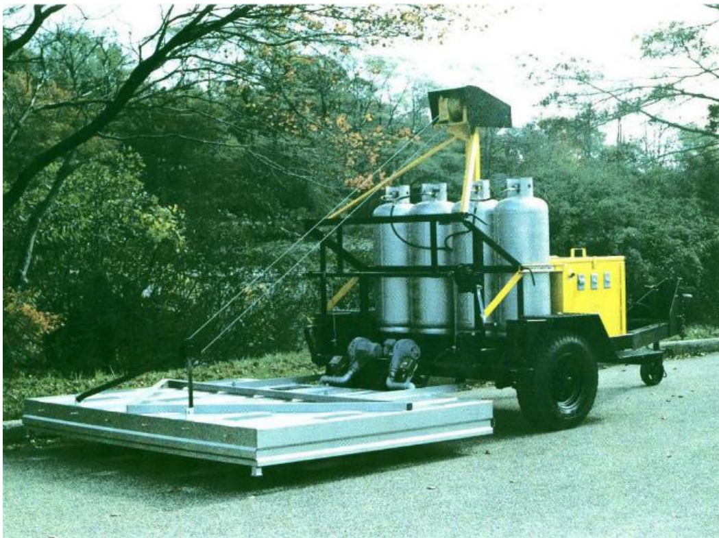
b. Heater Patching Trailer
