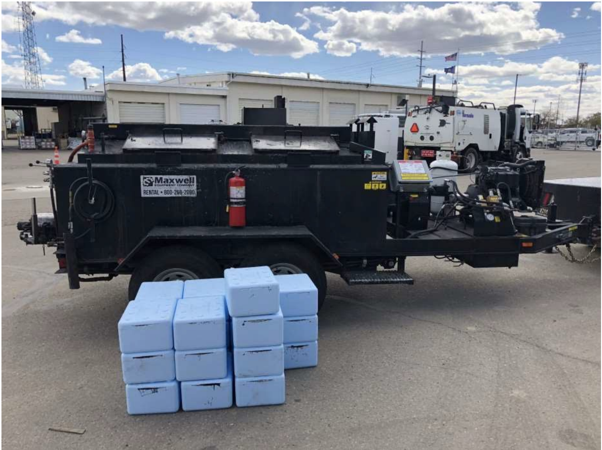
Figure 44. Material Blocks and Melter Kettle for Mastic Patch Material (Courtesy of Maxwell)
