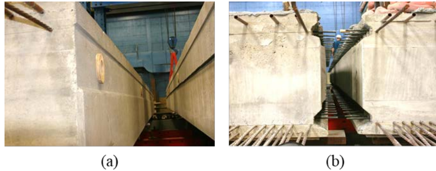
Figure 2.34: (a) Conventional shear key specimen and (b) UHPC shear key specimen [29]
