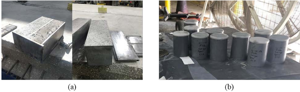
Figure 7.12: UHPC samples: (a) 4x4x14 in. beam in molds after grinding for dimensional consistency and (b) ten 4x8 in. cylinders for compressive strength
