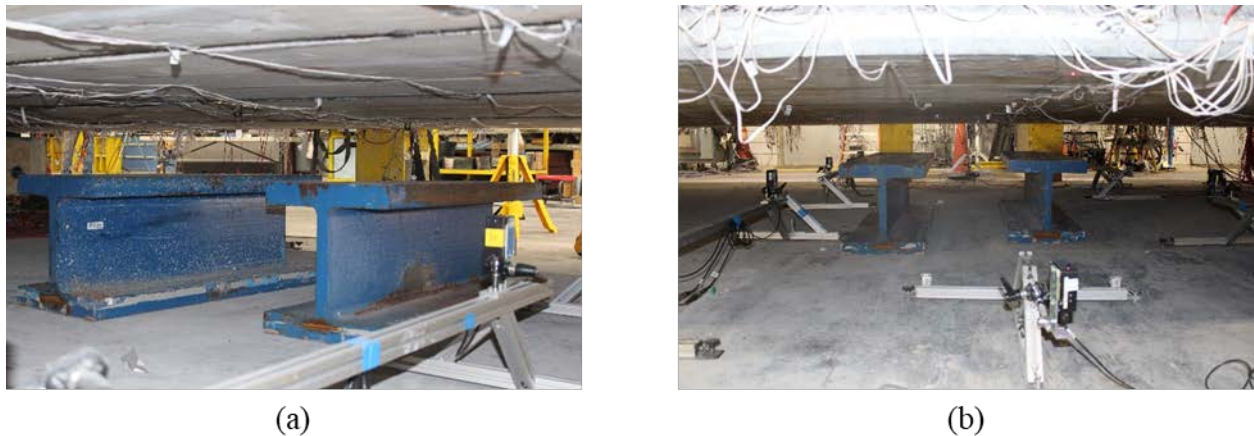
Figure 8.23: (a) Bottom steel I-beams, (b) clearance display between specimen and sensors
