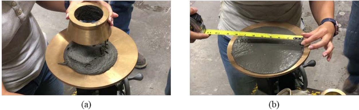
Figure 7.11: UHPC flow test: (a) mold removal and (b) spread measurement
