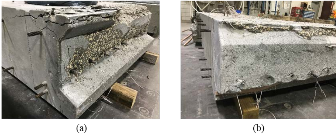
Figure 5.56: (a) Failed 18A1-1 specimen (loaded beam showed) and (b) UHPC matrix attached to unloaded beam
