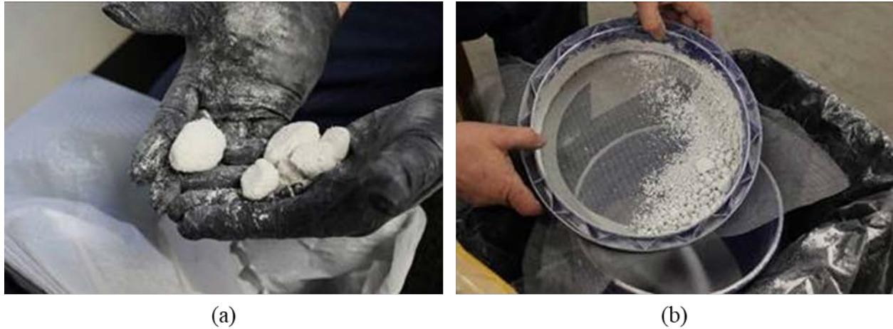
Figure 5.25: (a) Large and (b) small clumps collected from dry premix of UHPC
