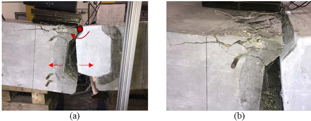
Figure D.25: 18A1-1: (a) failed specimen with complete UHPC matrix detachment, (b) Failure of top lip due to compressive stress concentration from west side
