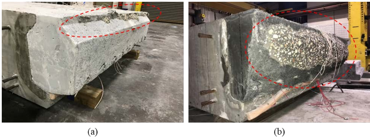
Figure 5.26: UHPC joint bond comparison: (a) poor bond observed with the faulty UHPC mixture and (b) enhanced bond observed with the adequate UHPC mixture
