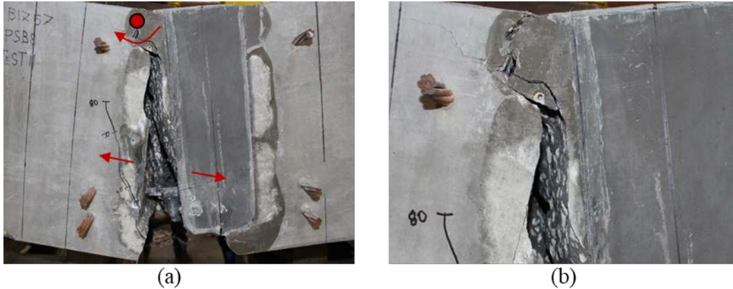
Figure D.21: 18F2-2: (a) possible tension and compression zones and (b) possible compressive stress concentration at the top in west side view
