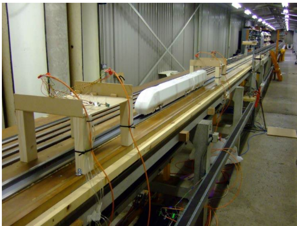
Figure 2-6. The “TRAIN rig” reduced-scale moving model testing facility in Derby, England, set up to measure pressure on a short overhead canopy; photo courtesy of Birmingham Centre for Railway Research and Education
