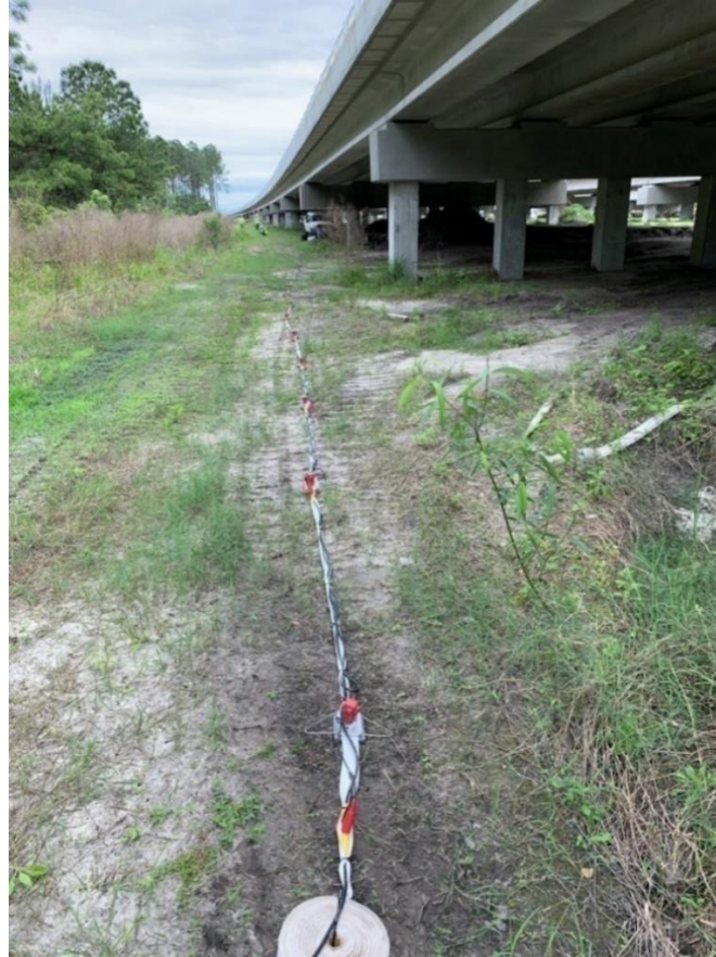
Figure 4.27. Wekiva Parkway, Bridge No. 110110, Bent 3 with problematic soils. A 70-m geophone array was used to record noise data and Bent 3 is at the middle of geophone array at distance of 35 m (117 ft).
